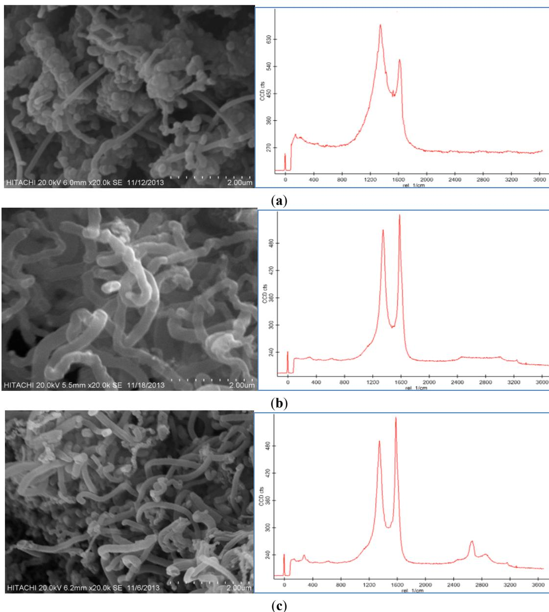
**Figure 3.** SEM images and Raman spectra of grown CNF by use of 100 mM catalyst concentration for 30 min under 50 sccm acetylene flow rate at (a) 450 °C, (b) 550 °C, and (c) 650 °C.
