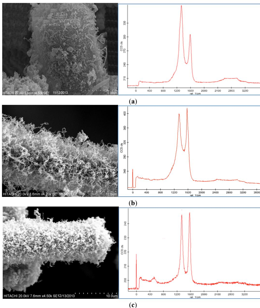
**Figure 5.** SEM images and Raman Spectrum of CNF morphologies at (a) 10 min, (b) 30 min, and (c) 50 min using 100 mM acid concentration at 550 °C under 50 sccm acetylene flow rate.
