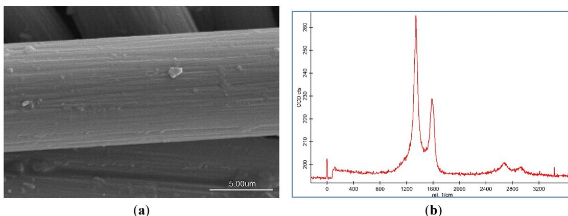
**Figure 1.** (a) Scanning electron microscopy (SEM) image; (b) Raman spectroscopy of pristine carbon fiber.
