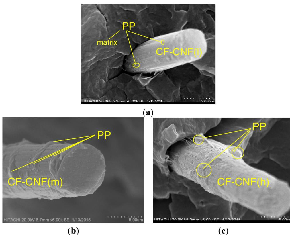
**Figure 9.** SEM micrographs of fractured surface of (a) CF-CNF<sub>L</sub>/PP, (b) CF-CNF<sub>M</sub>/PP, and (c) CF-CNF<sub>H</sub>/PP composites.
