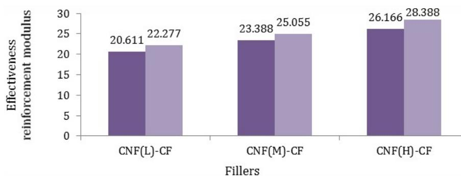
**Figure 8.** Effective reinforcement modulus of different fillers in polypropylene matrix (dark purple states minimum amount and light purple reveals maximum amount).
