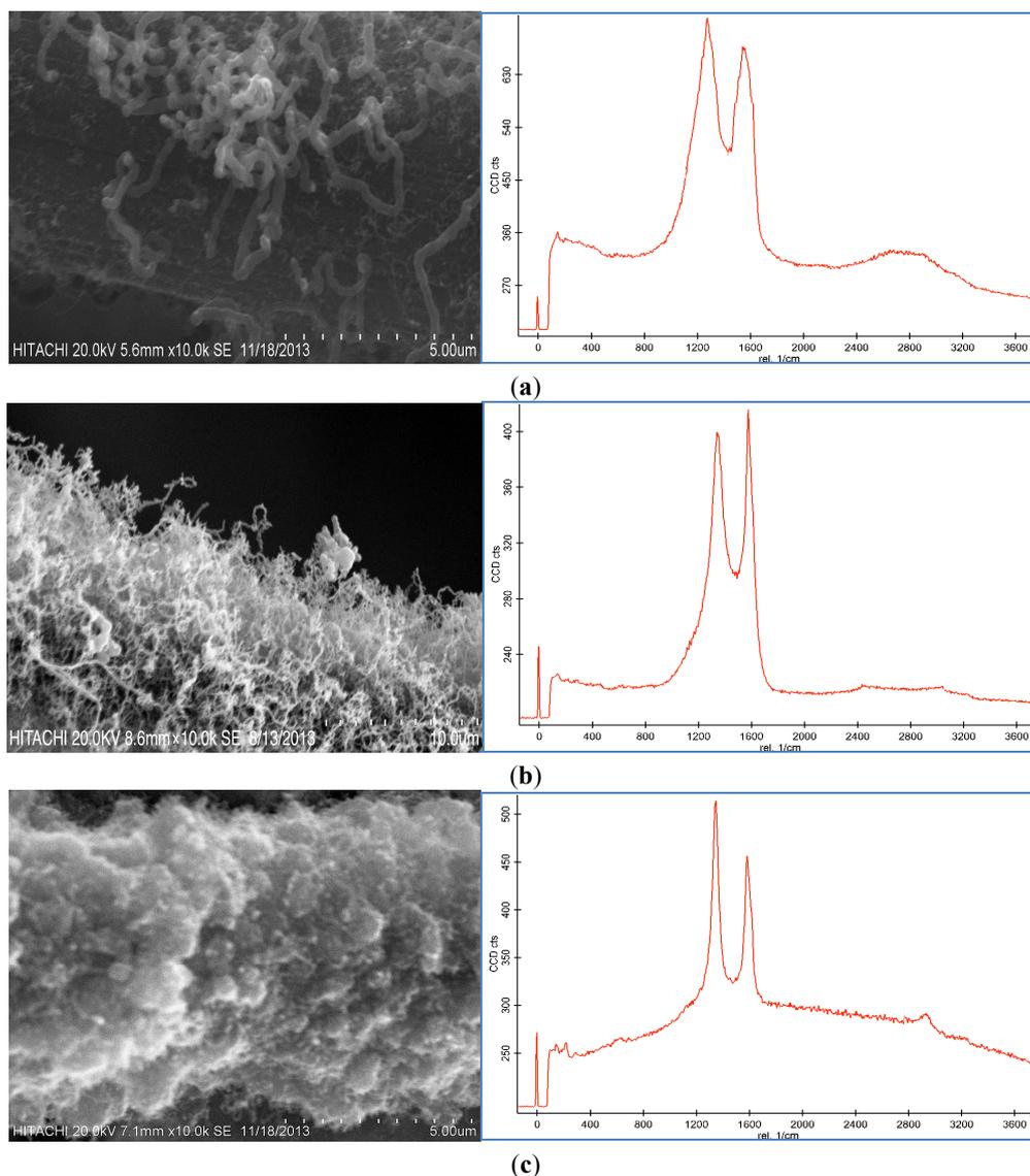
**Figure 2.** SEM images and Raman spectra of different agglomerations of grown carbon nanofibers (CNFs) on carbon fiber (CF) at (a) 50 mM, (b) 100 mM, and (c) 150 mM catalyst concentrations at 550 °C for 30 min run time under 50 sccm acetylene flow rate.
