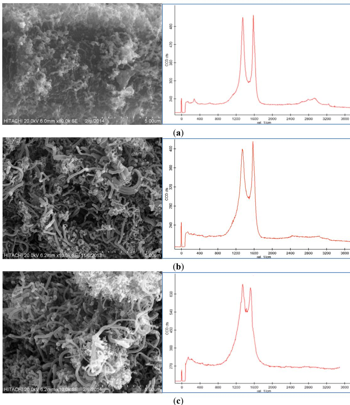
**Figure 6.** SEM images and Raman spectroscopy of carbon nanofiber on CF by use of 100 mM catalyst concentration at 550 °C for 30 min at (a) 25 sccm, (b) 50 sccm, and (c) 100 sccm flow rate of C<sub>2</sub>H<sub>2</sub>.
