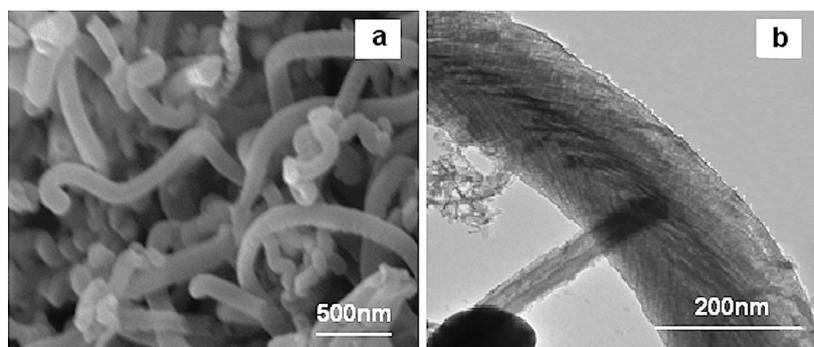
**Figure 7.** (a) SEM and (b) transmission electron microscopy (TEM) micrographs of optimum CNF.
