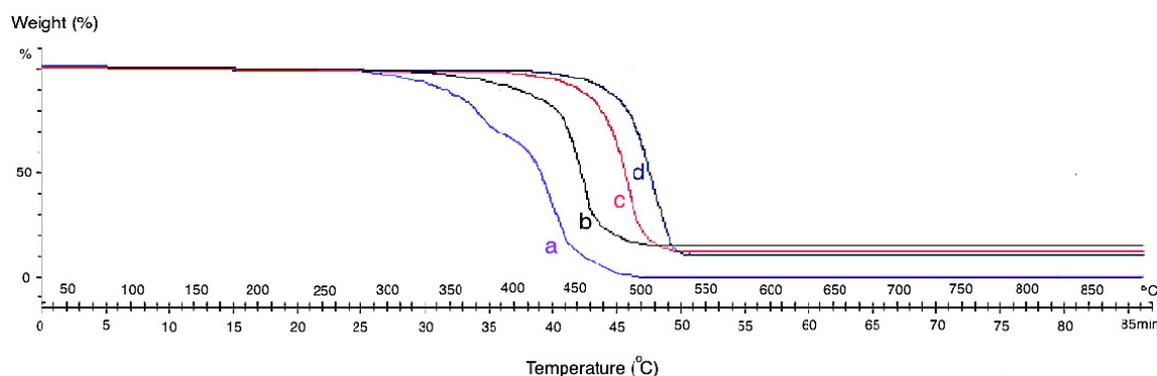
**Figure 4.** Themogravimetric analysis (TGA) analysis of (a) neat CF and CF-CNF at (b) 450 °C, (c) 550 °C, and (d) 650 °C.
