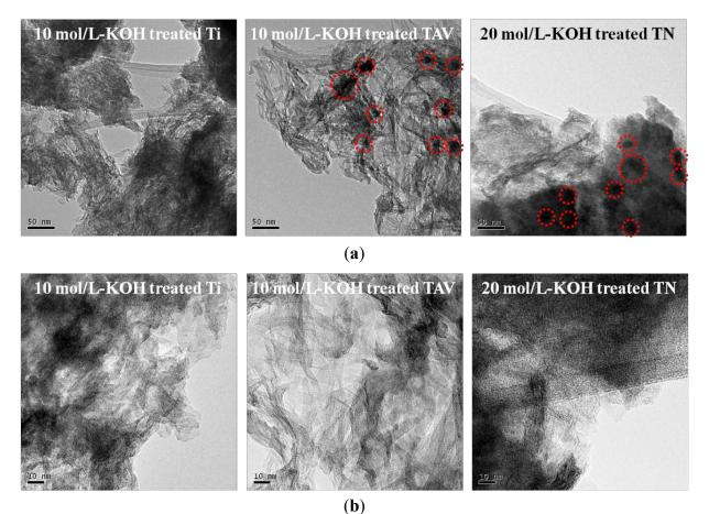
**Figure S1.** (**a**), (**b**) TEM images of microstructures of 10 mol/L-KOH treated Ti & TAV and 20 mol/L-KOH teated TN samples. TEM image show the similar layer structure of the nanowires within same morphology.
