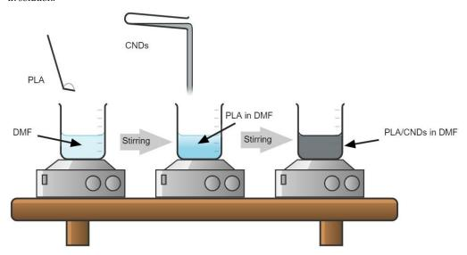
Figure 1. Preparation of solution for electrospinning.
