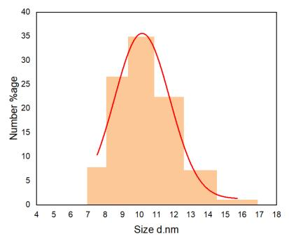
Figure 6. Size distribution of prepared CNDs measured by DLS.
