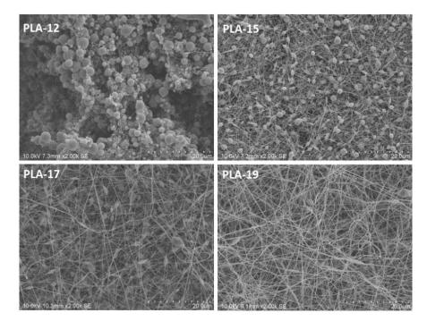
Figure 3. SEM images of pure PLA nanofibers with concentrations of 12, 15, 17, and 19% (scale— $20 \mu m$ ).
