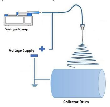
Figure 2. Electrospinning process for PLA nanofibers.
