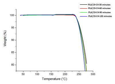
Figure 11. TGA analysis of PLA-19/C4 electrospun fibers.
