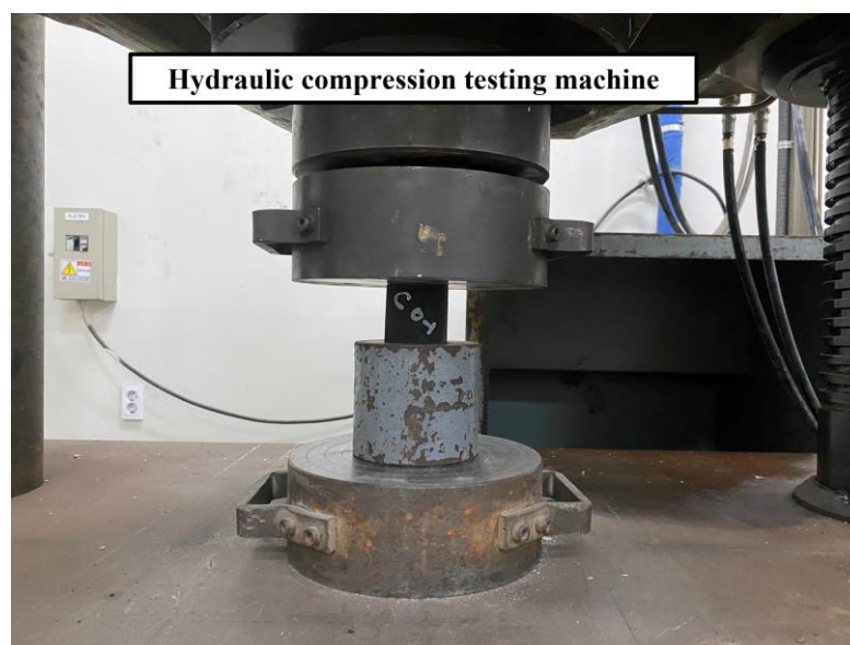
Figure 5. Compressive strength test set-up.
