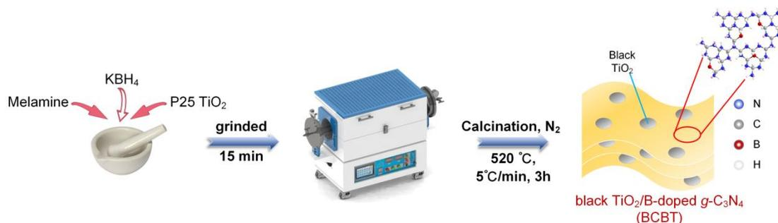
**Scheme 1.** Schematic illustration for synthesis of the black  $\text{TiO}_2$ /B-doped  $g\text{-C}_3\text{N}_4$  (BCBT).
