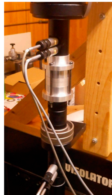
Figure 7. Four-microphone impedance tube for measuring transmission loss: (a) Schematic; (b) Photograph.
