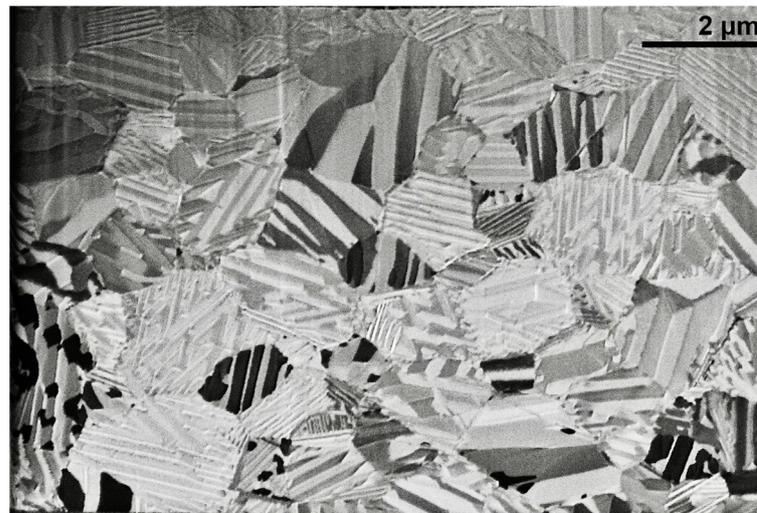
**Figure 5.** Focused Ga ions image taken on the FIB lamella, revealing the in-plane microstructure of the sample CAN/SN.
