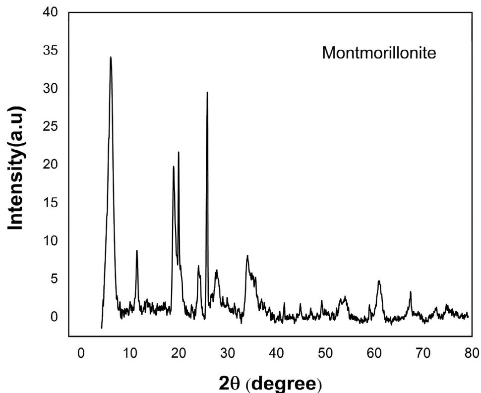
Figure 1. X-ray diffraction (XRD) graph of montmorillonite clay mineral.
