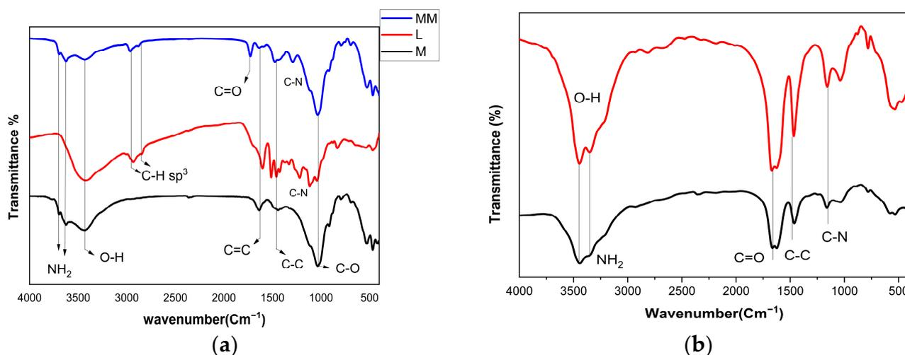
**Figure 3.** FTIR spectrum of: (a) lignin (red line), montmorillonite clay mineral (black line), and bio composite of lignin modified montmorillonite (blue line); (b) lignin/alginate/MMT biocomposite encapsulated urea (red line); alginate/urea (black line).
