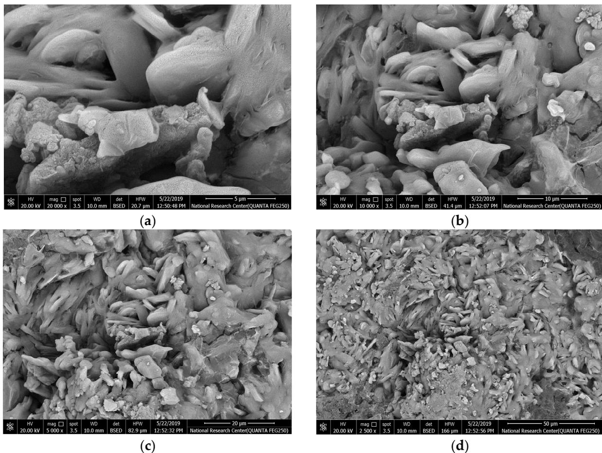
**Figure 4.** Scanning Electron Microscopy (SEM) images of lignin–montmorillonite bio-composite-based encapsulated urea (CRU beads) scanned at: (a) 20,000 $\times$ ; (b) 10,000 $\times$ ; (c) 5,000 $\times$ ; and (d) 2,500 $\times$  magnifications.
