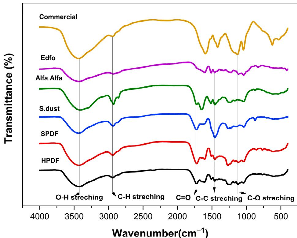
Figure 2. FTIR spectrograph of organosolv lignin; Alfa Alfa (green line), S. dust (blue line), Hard- (HDPF) and soft- (SDPF) date palm fibrillum (black and red lines, respectively). Alkaline ones, commercial (yellow line), and Edfo (purple line).
