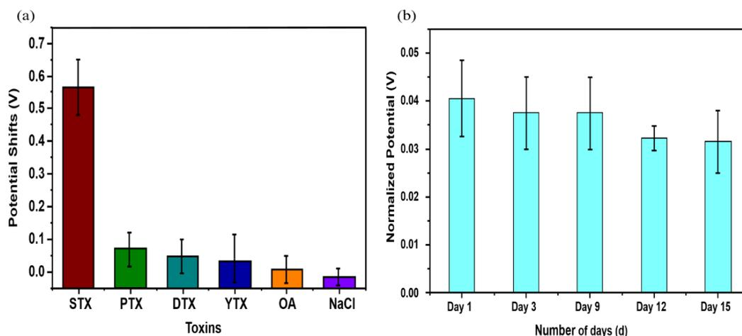
**Figure 6.** (a) Selectivity measurements of an aptasensor to STX (10 nM), DTX-1 (100 nM), PTX (100 nM), OA (100 nM), YTX (100 nM), and NaCl (100 nM). (b) Stability measurements of an aptasensor
