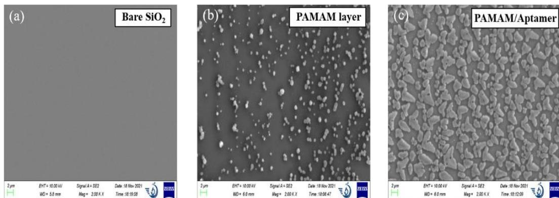
**Figure 1.** Characterization of biosensor preparation from a bare SiO<sub>2</sub> sensor surface. SEM images of (a) a bare sensor surface, (b) PAMAM dendrimer immobilization on a sensor surface, and (c) immobilization of Apt onto a PAMAM dendrimer-modified sensor surface.
