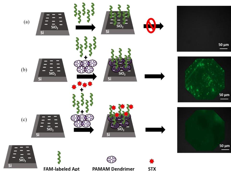
**Figure 3.** Schematic presentation and fluorescence images of (a) a bare sensor with FAM-labeled Apt solution, (b) FAM-labeled Apt incubated with PAMAM dendrimer-modified sensor surface, (c) STX solution incubated with PAMAM dendrimer/Apt-modified sensor.
