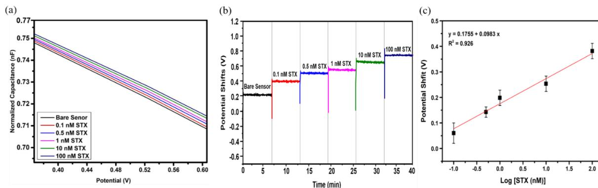
**Figure 5.** (a) C-V curves (b) ConCap analyses of an aptasensor in response to various STX concentrations of 0.5 nM to 100 nM. (c) Statistical results of ConCap analyses. All measurements were acquired in triplicates; error bars indicate standard deviation (SD).
