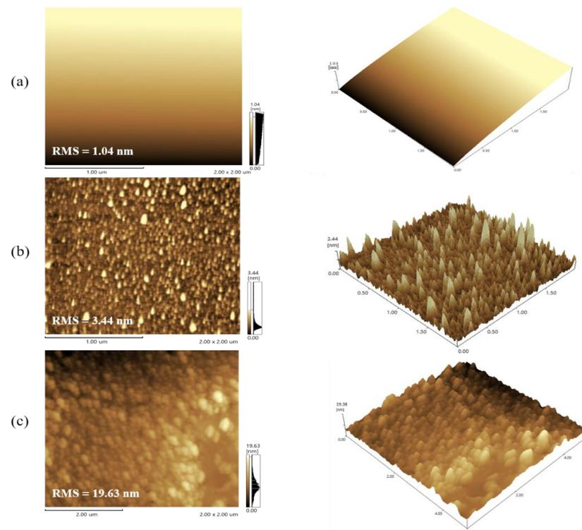
**Figure 2.** AFM characterization of biosensor preparation from bare SiO<sub>2</sub> sensor surface. (a) Bare sensor surface, (b) PAMAM dendrimer adsorption on a bare sensor surface, and (c) immobilization of Apt onto a PAMAM dendrimer-modified sensor surface.
