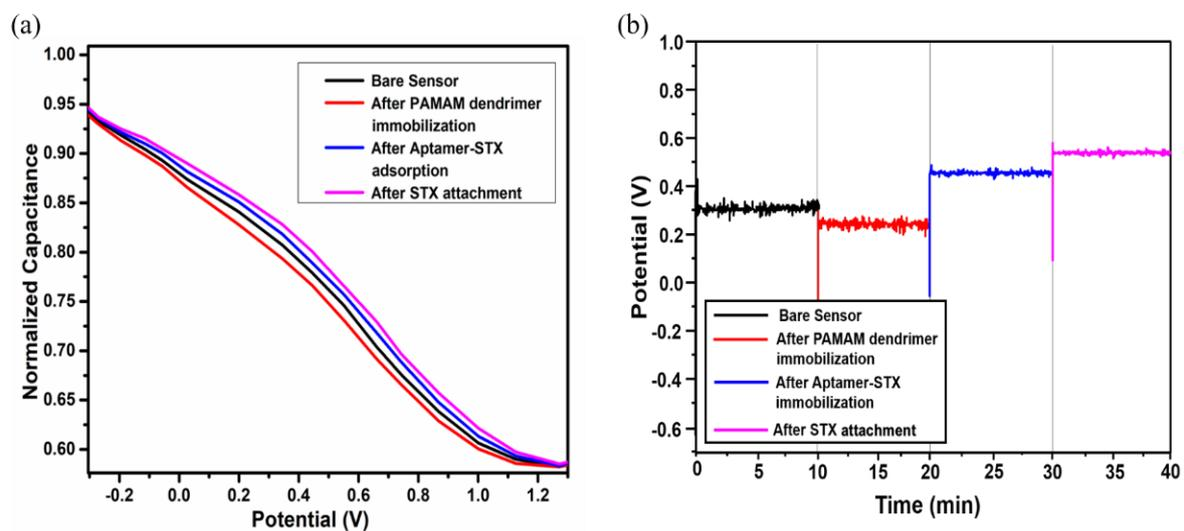
**Figure 4.** (a) C-V curves and (b) ConCap responses of a SiO<sub>2</sub> sensor recorded in a measurement solution before and after immobilization of PAMAM dendrimers, Apt, and after incubation with 100 nM STX. The working point for ConCap was set to 3.21 nF.
