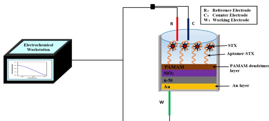
**Scheme 1.** Schematic measurement setup of a PAMAM dendrimer-modified EIS sensor with n-doped silicon, SiO<sub>2</sub> as gate insulator, and gold as a rear-side contact.
