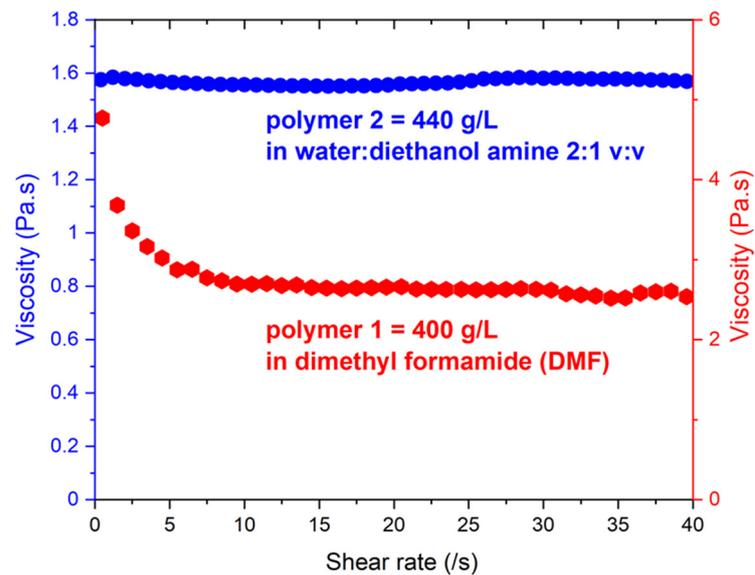
**Figure 2.** Viscosity of polymer solutions vs. shear rate (using polymer concentrations that correspond to electrospinning conditions, as shown in Table 1).
