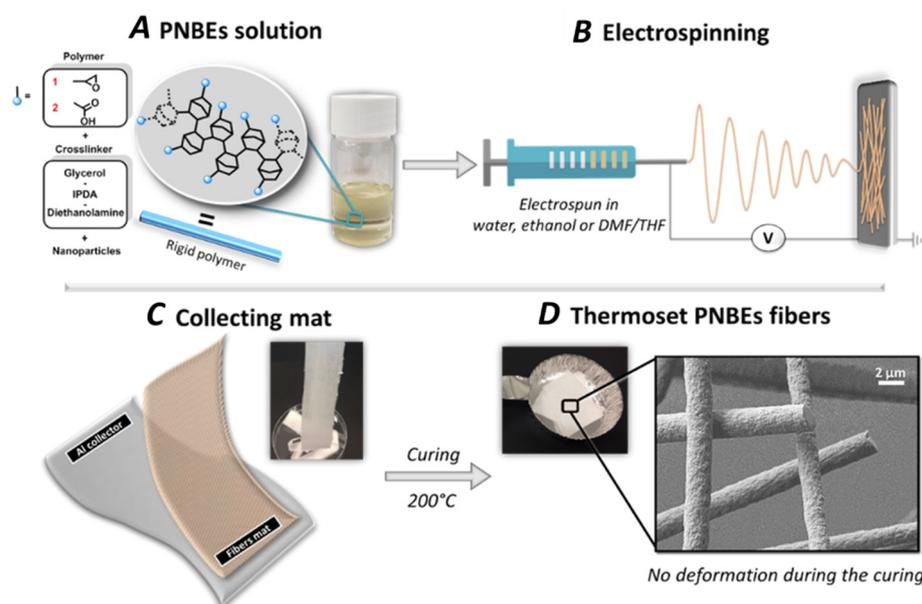
**Figure 1.** (A) Functional PNBE electrospun in this study; (B) schematic electrospinning process; (C) fibers collection process; (D) SEM image of the functional PNBE fibers after curing.
