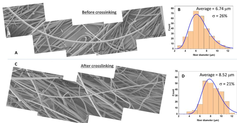
**Figure 4.** Assembled SEM pictures of fibers obtained by expt 1 (Table 1) before (A) and after (C) thermal treatment. The fiber that crosses all the images is approx 1 mm long. Each individual image has  $490 \times 220 \mu\text{m}$  dimension. Histogram of the fiber diameters measured on 150 fibers, measured before (B) and after (D) thermal treatment.
