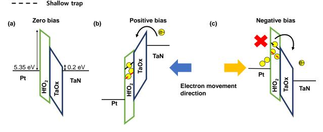
**Figure 4.** Band diagram schematic of PHTT device. (**a**) Zero bias condition. (**b**) Positive bias condition. (**c**) Negative bias condition.
