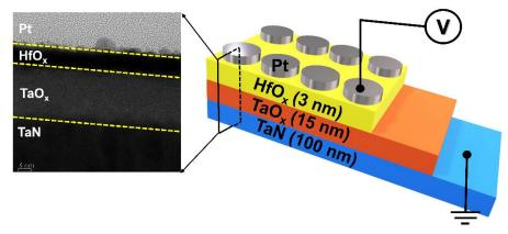
Figure 1. Cross-sectional TEM analysis and schematic of the Pt/HfO<sub>2</sub>/TaO<sub>x</sub>/TaN (PHTT3) device.
