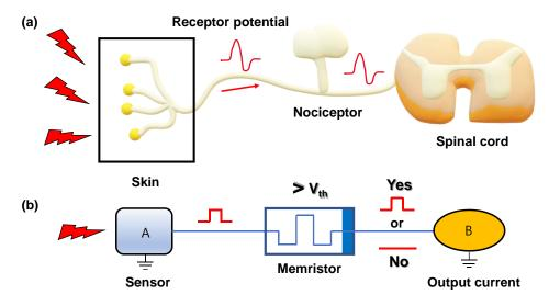
**Figure 2.** Nociceptor system in a human body and artificial nociceptor circuit using a TS memristor. (a) When external stimuli are introduced through the human skin, nociceptor determines the magnitude of the signal above the threshold and creates a potential to send information to the spinal cord. (b) Schematic in which an electrical pulse is applied to the sensor. A pulse higher than the threshold value is applied, the memristor is turned on and an output current is generated.
