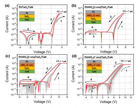
**Figure 3.** I–V characteristics of four devices: (**a**) PTT, (**b**) PHTT3, (**c**) PHTT5, (**d**) PHTT7. Schemes of the device are shown as the inset.
