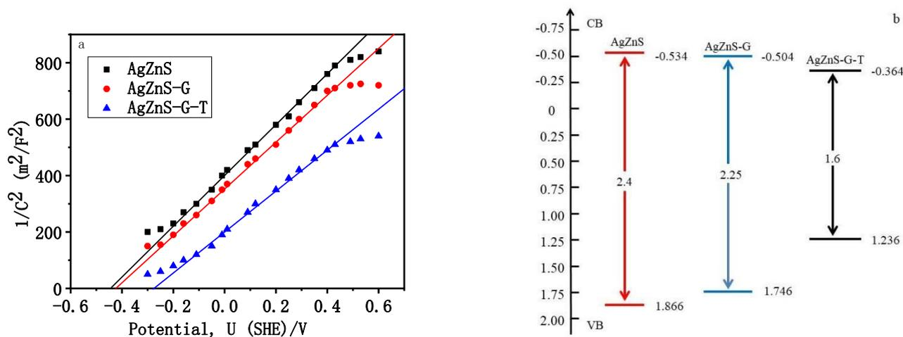
**Figure 6.** (a) Mott–Schottky analysis for calculation of donor density and flat band potential with 500 Hz frequency; (b) the band alignment of the prepared photocatalysts.
