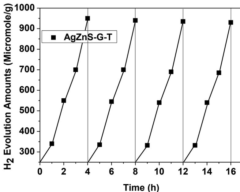
Figure 9. H<sub>2</sub> evolution of the circle test of AgZnS-G-T photocatalyst.
