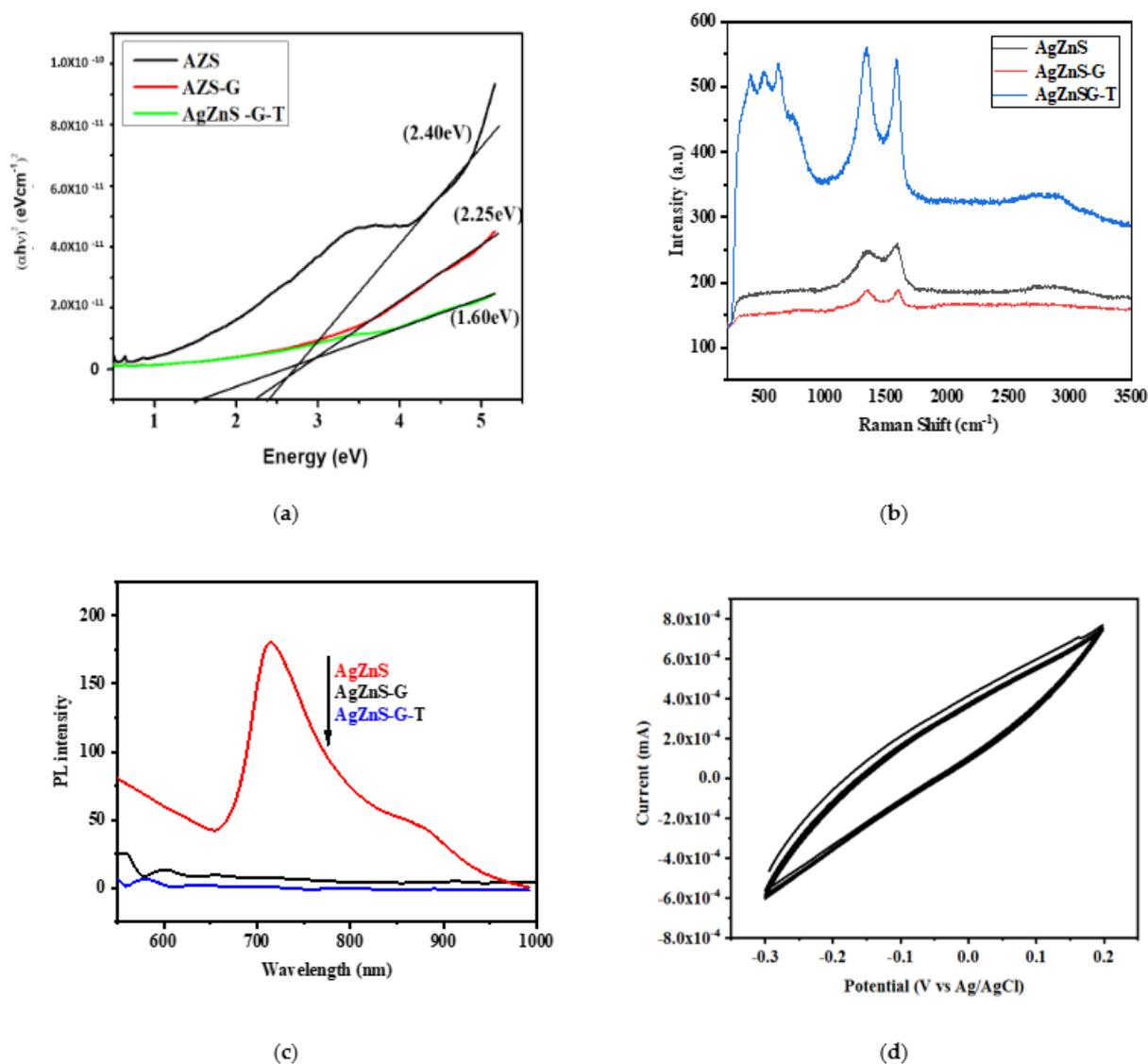
Figure 4. (a) UV-Vis DRS spectra; (b) RAMAN spectra; (c) PL spectra of AgZnS, AgZnS-G, and AgZnS-G-T photocatalysts; (d) cyclic voltammety of AgZnS-G-T photocatalysts.
