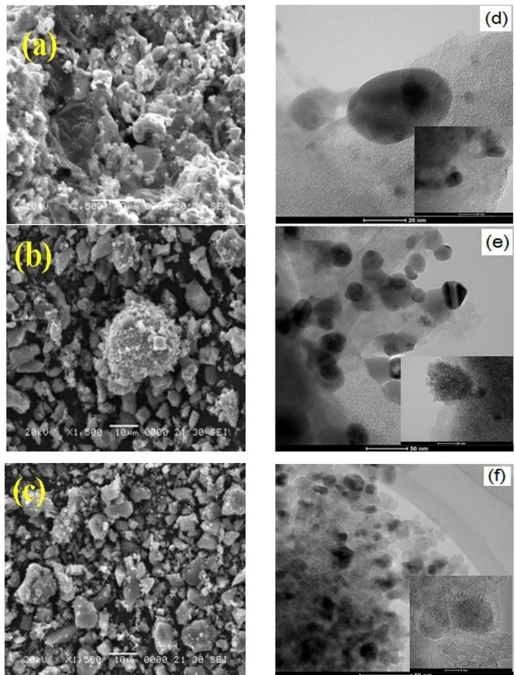
**Figure 2.** SEM images of (a) AgZnS; (b) AgZnS-G; (c,d) AgZnS-G-T photocatalysts. TEM images of (d) AgZnS; (e) AgZnS-G; (f) AgZnS-G-T samples.
