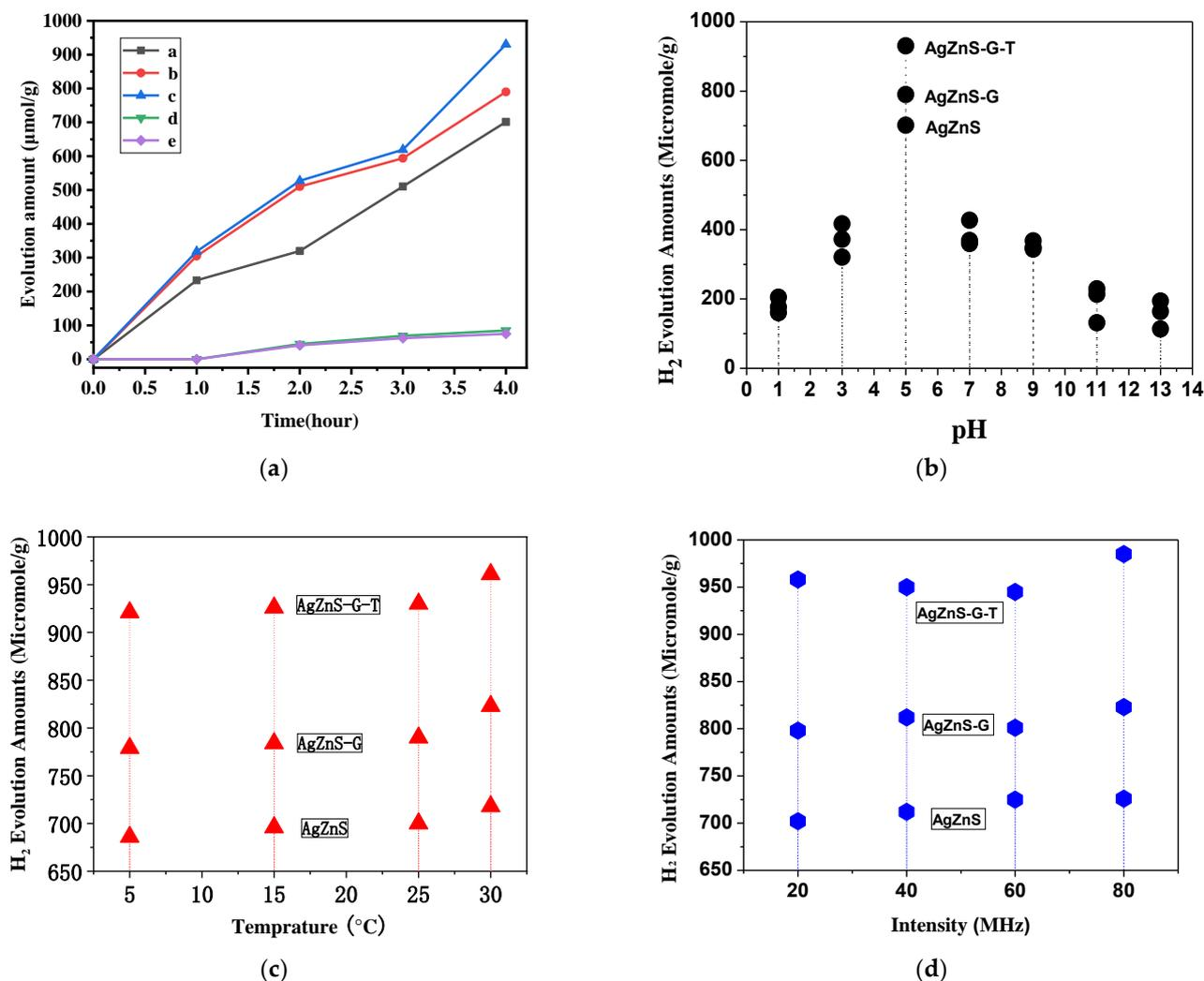
**Figure 7.** (a) Hydrogen evolution efficiency of a. AgZnS, b. AgZnS-G, c. AgZnS-G-T, d. GO, and e.  $\text{TiO}_2$  photocatalysts over time; (b) hydrogen evolution amount of AgZnS, AgZnS-G, and AgZnS-G-T photocatalysts with different pH condition; (c) with different temperature conditions; (d) with different ultrasonic intensity.
