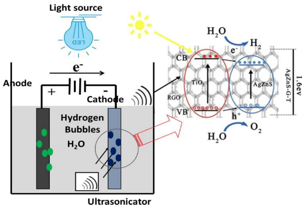
Figure 8. Electrosonophotocatalytic reduction and its mechanism of H<sub>2</sub> evolution on the electrode surface.
