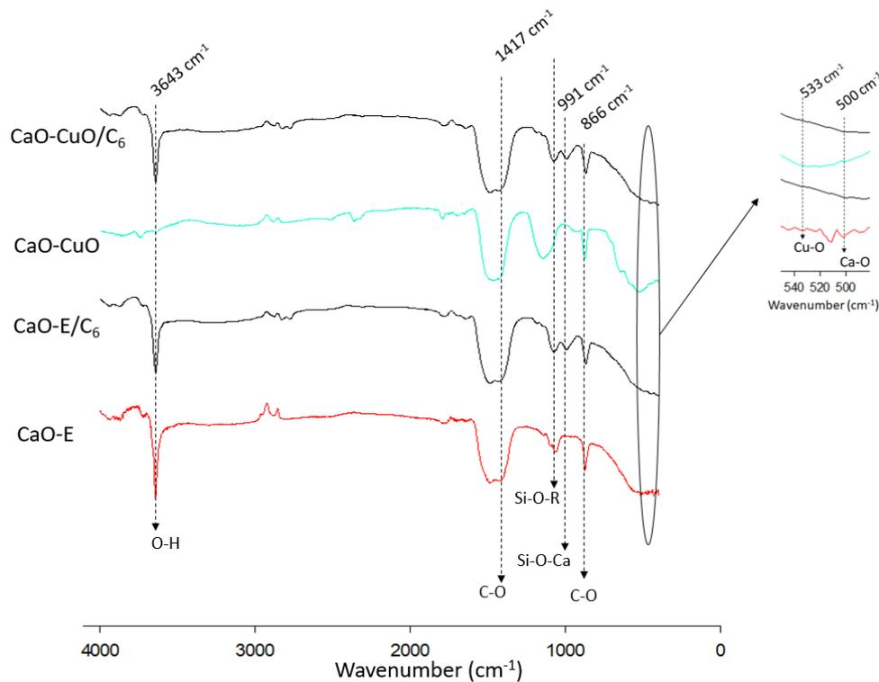
**Figure 3.** FTIR analysis of the catalyst: CaO-E, CaO-E/C<sub>6</sub>, CaO-CuO, CaO-CuO/C<sub>6</sub>.
