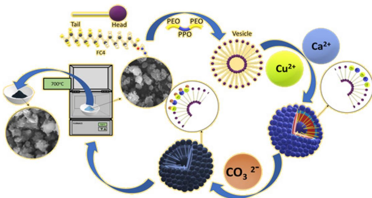
**Figure 1.** Synthesis of CaO-CuO by using the surfactant-controlled precipitation.
