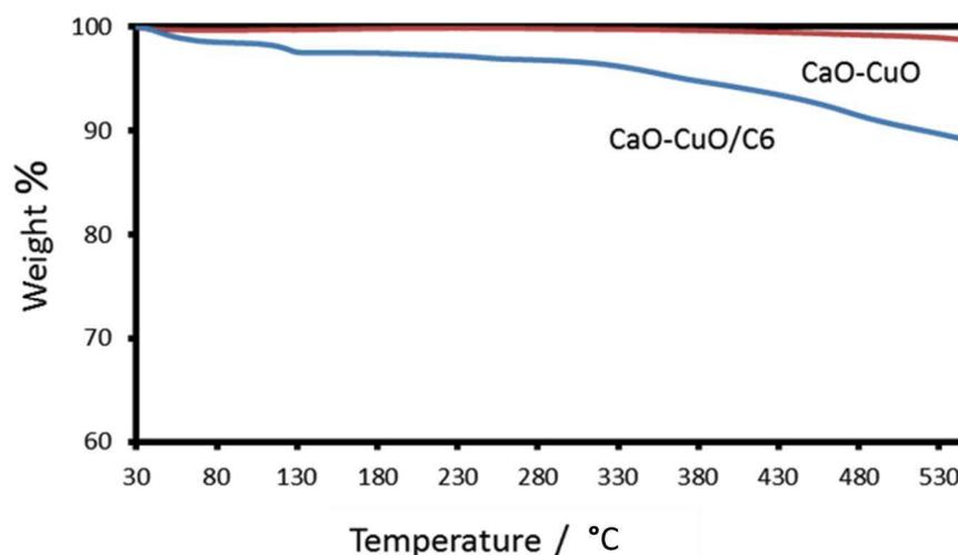
**Figure 4.** TGA analysis of the catalyst: CaO-CuO and CaO-CuO/C<sub>6</sub>.
