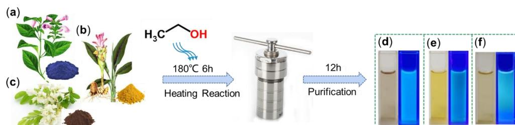
**Figure 1.** Schematic preparation of C-dots derived from natural plant dyes. (a–c) are the images of natural plants and dyes, corresponding to Indigo, *Carcuma longa*, and *Sophora japonica* L., respectively; (d–f) are C-dots solution upon room light (left) and 395 nm light illumination (right). The C-dots solutions were prepared via a heating reaction by using (d) Indigo, (e) *Carcuma longa*, and (f) *Sophora japonica* L. as precursors and ethanol as solvent.
