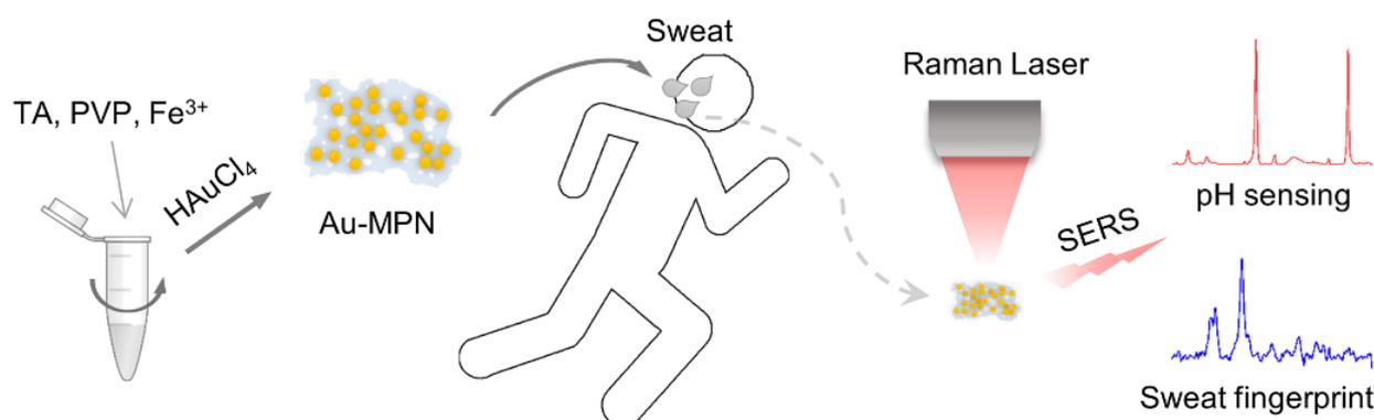
**Scheme 1.** Illustration of the MPN-based SERS substrate and its application for sweat sensing.
