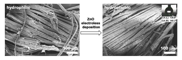
**Figure 5.** FESEM images of flax and ZnO-coated flax fibers as fabrics. In the inset is shown the optical photograph of the water droplet shape on the hydrophobic surface of ZnO-coated flax fabrics and the water contact angles for the corresponding sample.
