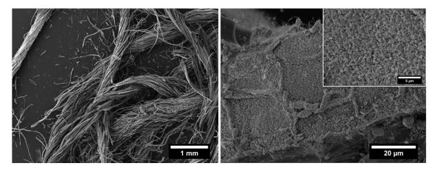
**Figure 8.** FESEM images at different magnifications of ZnO-coated flax yarns after the thermogravimetric test.
