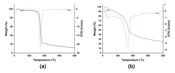
**Figure 7.** TGA (black solid curves) and dTG (red dot curves) thermograms of (**a**) neat flax yarns and (**b**) ZnO-coated flax yarns (arrows indicate the corresponding Y axis).
