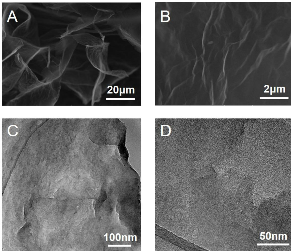
**Figure 2.** Characterizations of the surface morphology of graphene. (A,B) SEM images of graphene and (C,D) TEM images of graphene.
