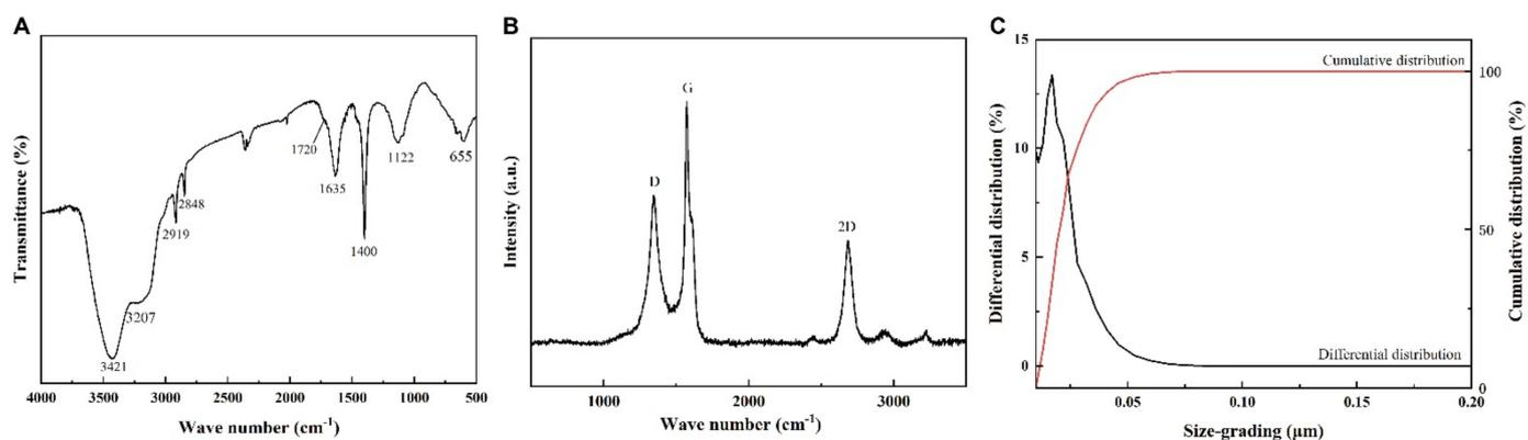
**Figure 3.** Composition and structure analyses of graphene. (A) FT-IR spectra of graphene, (B) Raman spectra of graphene, and (C) size distribution of graphene.
