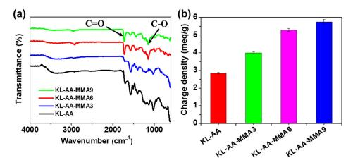
**Figure 3.** (a) FTIR spectra (4000–600 cm $^{-1}$ ) and (b) charge density of KL-AA and KL-AA-MMA copolymers.
