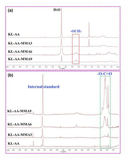
Figure 2. (a) <sup>1</sup>H-NMR and (b) <sup>31</sup>P-NMR spectra of the KL-AA and KL-AA-MMA copolymers.
