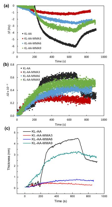
**Figure 5.** (a) Frequency and (b) dissipation at the third overtone for the adsorption of KL-AA and KL-AA-MMA nanoparticles on xylene-coated  $SiO_2$  sensors. (c) thickness growth over time for KL-AA and KL-AA-MMA nanoparticles obtained via the Voigt model.
