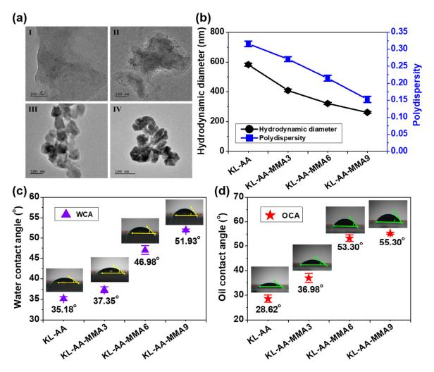
**Figure 4.** (a) TEM images of (I) KL-AA, (II) KL-AA-MMA3, (III) KL-AA-MMA6, and (IV) KL-AA-MMA9 nanoparticles. (b) Hydrodynamic diameter and polydispersity, (c) water and (d) oil contact angles of various KL-AA-MMA nanoparticles.
