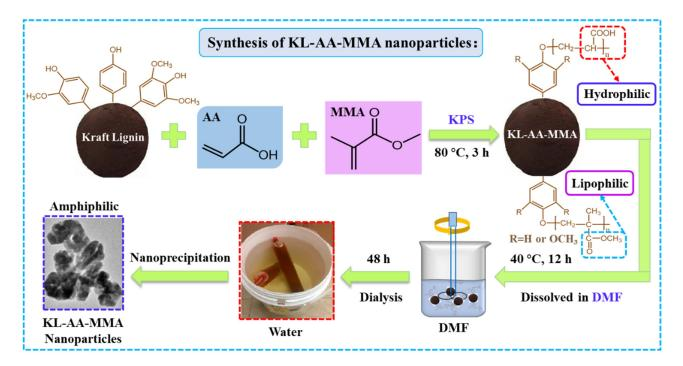
Figure 1. Schematic illustration for the synthetic process of KL-AA-MMA nanoparticles.
