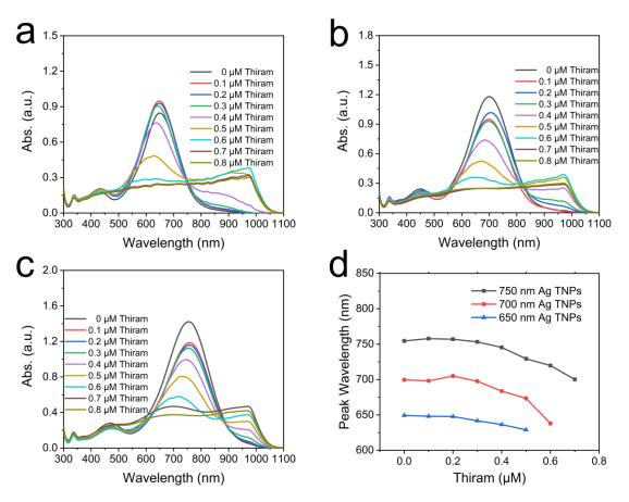
**Figure 6.** The absorption spectra of the Ag TNPs with main absorption peaks at 650 nm (**a**), 700 nm (**b**), and 750 nm (**c**) after adding different concentrations of thiram. The peak positions change the trend with the concentration of thiram increasing (**d**).
