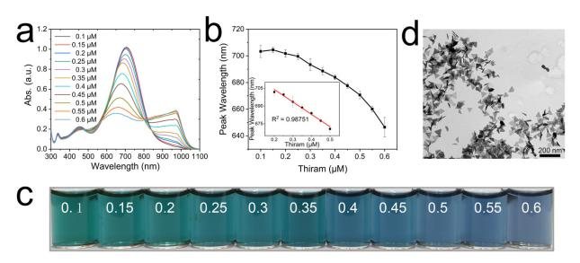
**Figure 7.** Ag TNPs-based detection of thiram. The absorption spectra of Ag TNPs by adding different concentrations of thiram (**a**). The curve of the main absorption peak shift with the concentration of thiram (**b**), the inset in (**b**) is the linear fitting results. The digital photograph corresponding to the above samples (**c**). The cryo-TEM image of the Ag TNPs with 0.6  $\mu$ M of thiram (**d**).
