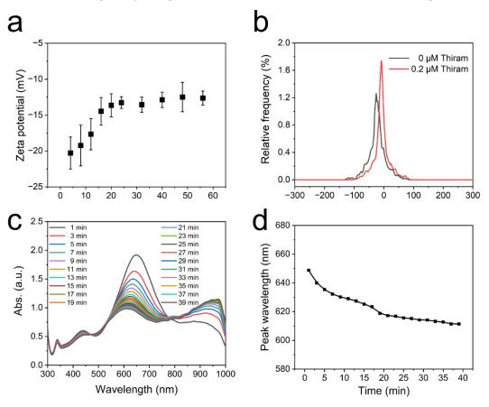
**Figure 1.** Zeta potential change trend with time by adding 0.2  $\mu$ M of thiram (**a**). Zeta potentials of the Ag TNPs solution before and after adding thiram (**b**). The absorption spectra (**c**) and the peak wavelength change trend of the main absorption peak (**d**) with time by adding 0.3  $\mu$ M of thiram into the Ag TNPs (the main absorption peak of the original Ag TNPs is located at 650 nm).
