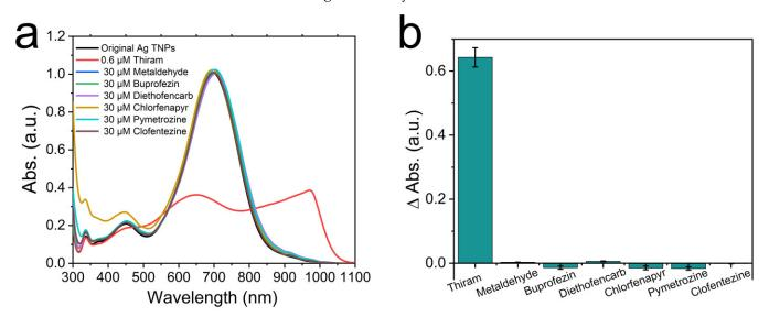
**Figure 8.** The selectivity of this method for detection of thiram. The absorption spectral characteristics (**a**) and the main absorption peak position changes (**b**) of the samples by adding thiram (0.6  $\mu$ M) and other interfering pesticides (30  $\mu$ M) relative to the sample without any pesticides, respectively.
