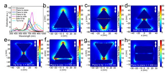
**Figure 3.** The extinction spectra of the monomer and the six assembly forms of Ag TNPs (the polarization was set to both along and perpendicular to the coupling direction) (**a**). The LEF distributions of the monomer (**b**) and the six assembly forms (**c**–**h**) of Ag TNPs (the polarization was set along the coupling direction, as shown by the arrow in the figures).
