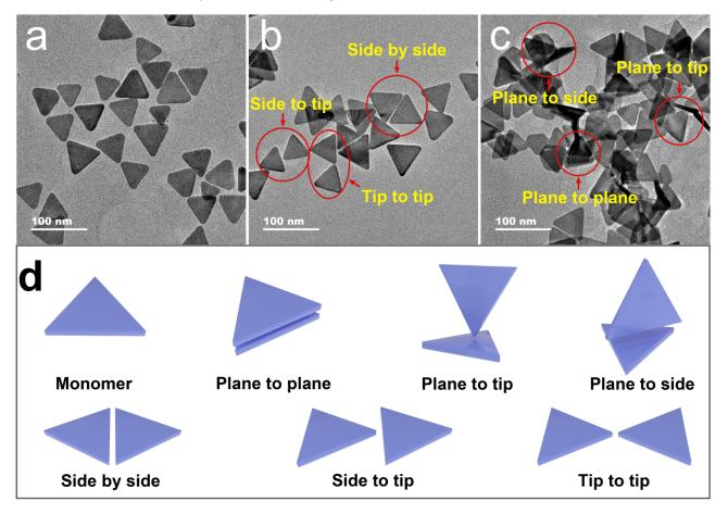
**Figure 2.** The TEM images of the Ag TNPs with the main absorption peak at 700 nm after adding different concentrations of thiram. The TEM images of the Ag TNPs with 0  $\mu$ M (**a**), 0.4  $\mu$ M (**b**), and 0.6  $\mu$ M (**c**) of thiram. The schematic diagrams of different assembly forms of the stabilizer-removal induced Ag TNPs aggregates (**d**).
