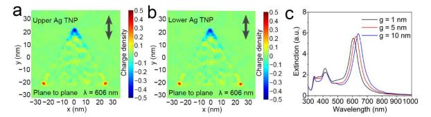
**Figure 4.** The charge distributions of the upper (**a**) and lower (**b**) Ag TNP in plane-to-plane form (the polarization was shown by the arrow in the figures). The extinction spectra of the plane-to-plane form of Ag TNPs with different gap values g (the polarization was set to both along and perpendicular to the coupling direction) (**c**).
