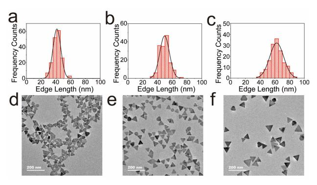
**Figure 5.** The histograms of the size distribution of the Ag TNPs with main absorption peaks at 650 nm (**a**), 700 nm (**b**), and 750 nm (**c**). The low magnification TEM images of the Ag TNPs with main absorption peaks at 650 nm (**d**), 700 nm (**e**), and 750 nm (**f**).
