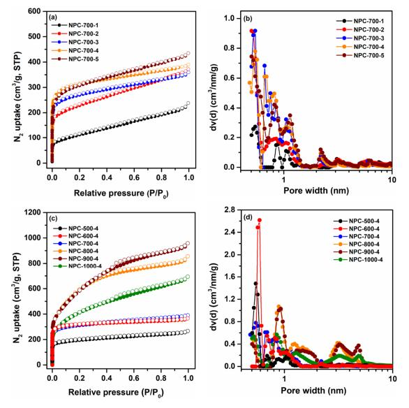
**Figure 7.** 77 K N<sub>2</sub> adsorption (filled) and desorption (empty) isotherms (**a**,**c**) and pore size distributions (**b**,**d**) of NPC-700-x and NPC-y-4.
