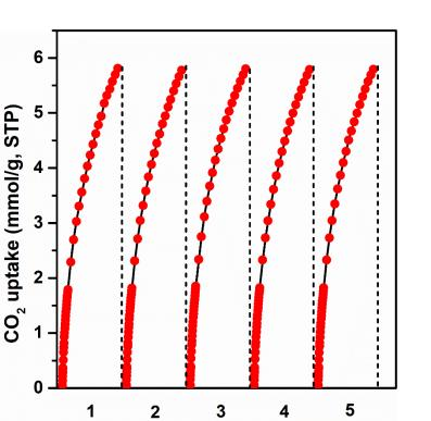
Figure 12. Five consecutive adsorption-desorption cycles of NPC-600-4 at 273 K.
