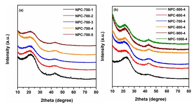
Figure 5. X-ray diffraction patterns of NPC-700-x (a) and NPC-y-4 (b).
