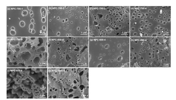
Figure 4. SEM images of NPC-700-x (a-e) and NPC-y-4 (f-j).
