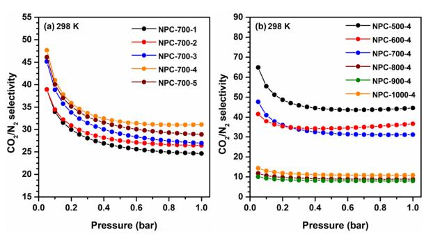
Figure 11. IAST  $CO_2/N_2$  adsorption selectivity of NPC-700-x (a) and NPC-y-4 (b) at 298 K.
