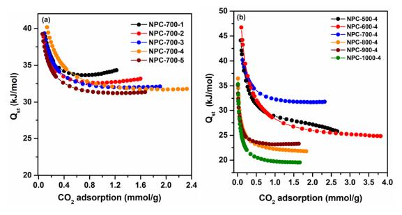
Figure 9. Isosteric heat of CO<sub>2</sub> adsorption as a function of CO<sub>2</sub> uptake for NPC-700-x (a) and NPC-y-4 (b).
