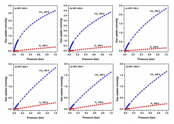
Figure 10. CO<sub>2</sub> and N<sub>2</sub> adsorption isotherms of NPC-y-4 (a-f) at 298 K.
