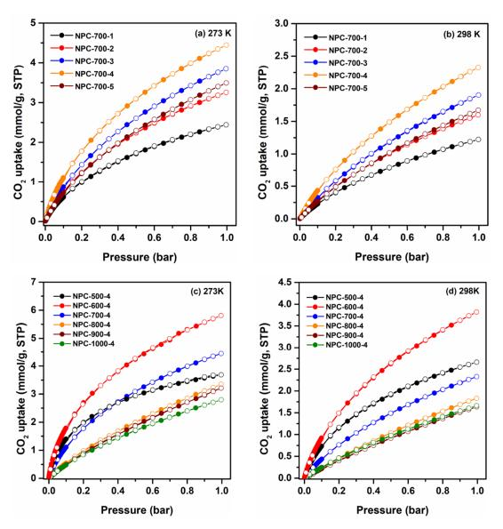
Figure 8. CO<sub>2</sub> adsorption-desorption isotherms at 273 K and 298 K for NPC-700-x (a,b) and NPC-y-4 (c,d).
