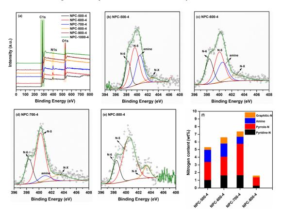
**Figure 2.** XPS (**a**), N1s XPS (**b**–**e**) spectra of NPC-y-4, and the contents of the nitrogen group in NPC-y-4 (**f**).
