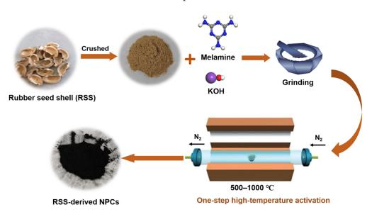
Scheme 1. Synthetic illustration of the synthesis of RSS-based NPCs.
