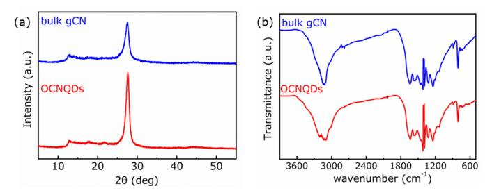
Figure 3. (a) The XRD diagrams; (b) the FT-IR spectra of bulk gCN and OCNQDs.
