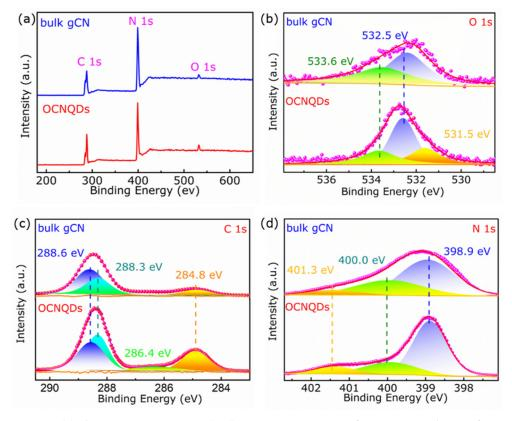
**Figure 4.** (a) The survey XPS spectra; (b–d) narrow scan spectra of O 1s, C 1s, and N 1s of OCNQDs and bulk gCN.
