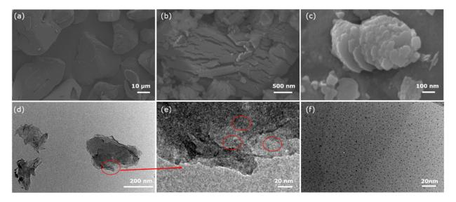
**Figure 1.** The SEM images of (**a**) melamine, (**b**) melamine precursor, (**c**) bulk O-gCN; the TEM images of (**d**) O-gCN nanosheets, (**e**) the edge of O-gCN nanosheets at higher magnification, (**f**) OCNQDs.
