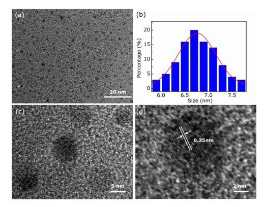
Figure 2. (a) TEM image, (b) particle size distribution analysis, (c,d) HRTEM images of OCNQDs.
