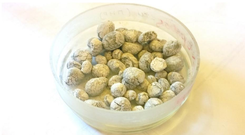
**Figure 2.** Granules of unsintered sorbent.
