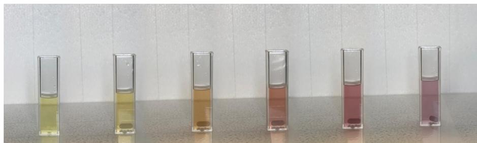
Figure 7. Color changes of AgNPs@11MUA upon addition of increasing concentration of Ni<sup>2+</sup>.
