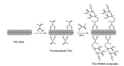
**Figure 5.** Schematic of functionalization of  $TiO_2$  and formation of  $TiO_2$ -PMMA nanocomposite. Reproduced from Ref. [85] with permission from the ACS, 2007.
