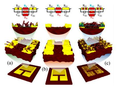
**Figure 13.** Models and equivalent circuit of the submicron-rod (**a**), thin film (**b**) and submicron-tree (**c**) sensors. It is noted that the total resistance will be reduced if  $R_R$  and  $R_{BR}$  decrease upon exposure to  $H_2S$ . Reproduced from Ref. [116] with permission from Elsevier, 2014.
