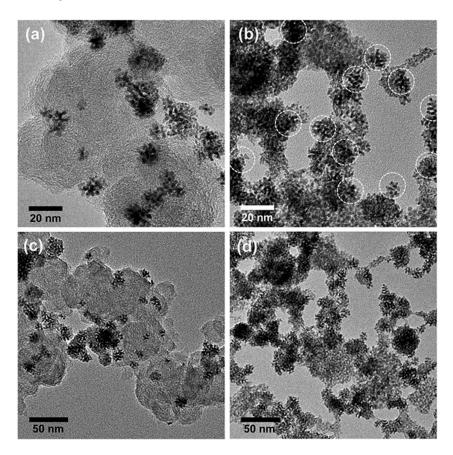
**Figure 14.** HR-TEM images of Ir-nanodendrite supported on (a) carbon black and (b) antimonydoped tin oxide. Low magnification TEM images of (c) Ir-nanodendrite/carbon and (d) Ir-nanodendrite/antimony-doped tin oxide. Reproduced from Ref. [20] with permission from the Royal Society of Chemistry, 2015.
