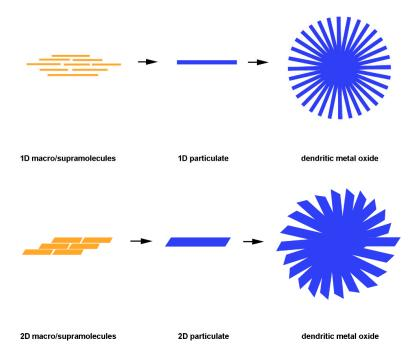
**Scheme 1.** Dendritic metal oxides are organized 1D or 2D particulates in certain patterns. The particulates are composed of 1D or 2D macromolecules/supramolecules.
