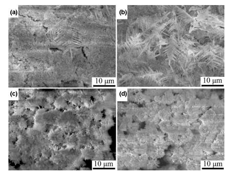
**Figure 3.** SEM images of SnO<sub>2</sub> leaf-like microstructure with different amounts of diammonium phosphate (a) 0.15 g, (b) 0.2 g, (c) 0.22 g, (d) 0.25 g. Reproduced from Ref. [62] with permission from Elsevier, 2018.
