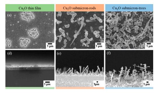
**Figure 12.** Top-view and cross-section FE-SEM images of  $Cu_2O$  thin film  $(\mathbf{a},\mathbf{d})$ , submicron-rods  $(\mathbf{b},\mathbf{e})$  and submicron-trees  $(\mathbf{c},\mathbf{f})$ . Reproduced from Ref. [116] with permission from Elsevier, 2014.
