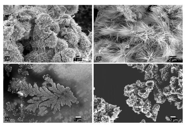
**Figure 2.** SEM images of  $TiO_2$  dendritic nanostructures prepared via sol-gel reactions of titanium isopropoxide with acetic acid in  $scCO_2$  (a,b) and isopropanol (c,d).
