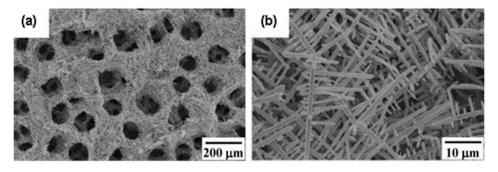
**Figure 4.** SEM images at two different magnifications (**a**) and (**b**) for Sn foams synthesized from electrochemically deposition after 15 s. Reproduced from Ref. [78] with permission from Elsevier, 2012.
