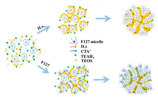
**Figure 7.** Mechanism for the synthesis of dendritic mesopores within silica nanoparticles with controllable particle size. Reproduced from Ref. [93] with permission from the ACS, 2014.
