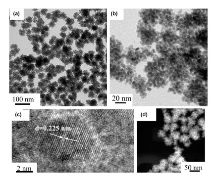
**Figure 15.** TEM images of Pd nanodendrites at different magnification (**a**,**b**); (**c**) HR-TEM image of Pd nanodendrites; (**d**) ADF-STEM image of Pd nanodendrites. Reproduced from Ref. [134] with permission from the ACS, 2009.
