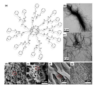
**Figure 6.** Chemical structure of a polyhedral oligomeric silsesquioxane core-based dendrimer (a). Stacking of this planar structure would form a linear structure which grows in the direction out of this paper. TEM (b,c) and SEM (d–g) images of the xerogel obtained in methyl methacrylate solvent under different magnifications. The red cycles highlight the areas where a higher magnification image was taken. Reproduced from Ref. [90] with permission from the ACS, 2017.
