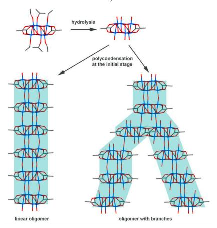
**Figure 8.** Hydrolysis and polycondensation of  $T_{i_6}O_6(OAc)_6(O^iPr)_6$  can form linear or branched oligomers at the initial stage of sol-gel reactions. These oligomers may grow into agglomerated 1D and dendritic nanostructures in  $scCO_2$ . Note:  $T_i = blue$ ; O = red; C = dark gray; H atoms omitted for clarity.
