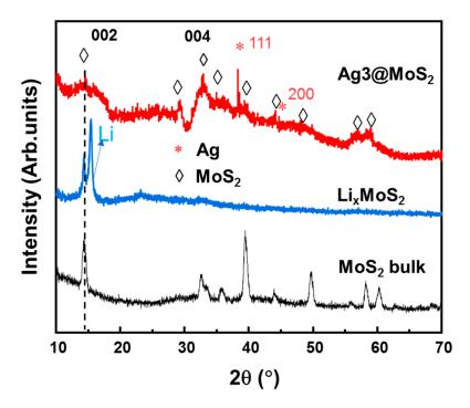
Figure 2. X-ray diffraction patterns of bulk MoS<sub>2</sub>, Li<sub>x</sub>MoS<sub>2</sub>, and Ag3@MoS<sub>2</sub> materials.
