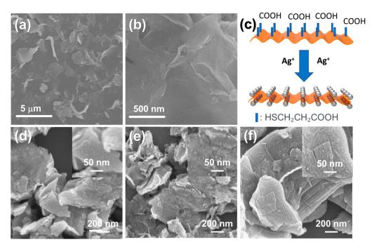
**Figure 1.** (a,b) Scanning electron microscopy (SEM) images of MoS<sub>2</sub> nanosheets (NSs); (c) illustration of Ag-decorated MoS<sub>2</sub> NS; SEM images of (d) Ag1@MoS<sub>2</sub>, (e) Ag2@MoS<sub>2</sub>, and (f) Ag3@MoS<sub>2</sub> NSs.
