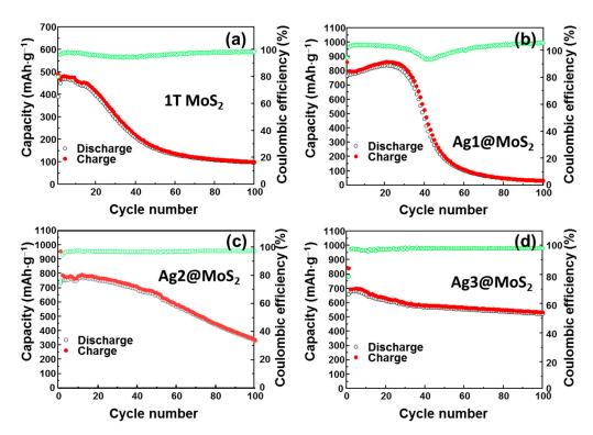
Figure 6. Cyclic performance of (a) MoS<sub>2</sub> NSs, (b) Ag1@MoS<sub>2</sub>, (c) Ag2@MoS<sub>2</sub>, and (d) Ag3@MoS<sub>2</sub> anodes.
