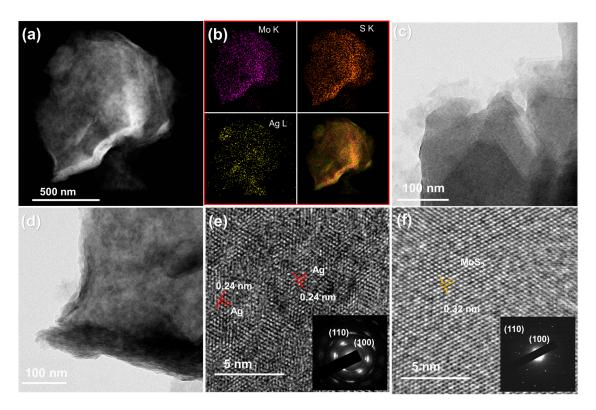
**Figure 3.** (a,b) Transmission electron microscopy (TEM) image and element mapping images of Ag3@MoS<sub>2</sub> materials; (c,f) TEM, high-resolution TEM (HRTEM) with inset selected area electron diffraction (SAED) pattern of MoS<sub>2</sub> NS; (d,e) TEM, HRTEM with inset SAED pattern of Ag3@MoS<sub>2</sub> materials.
