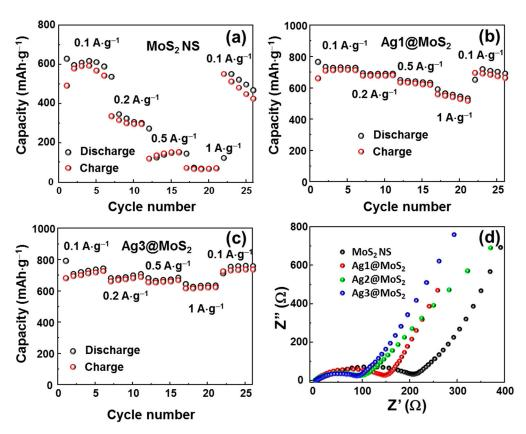
**Figure 7.** Rate performance of (**a**) MoS<sub>2</sub> NSs, (**b**) Ag1@MoS<sub>2</sub>, (**c**) Ag3@MoS<sub>2</sub>, and (**d**) Nyquist plots of MoS<sub>2</sub> without/with Ag-decorated anodes.
