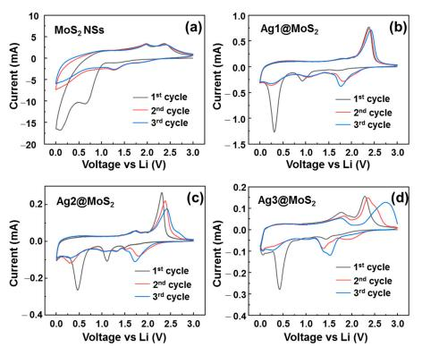
**Figure 4.** Cyclic voltammetry (CV) profiles of (a)  $MoS_2$  NSs, (b)  $Ag1@MoS_2$ , (c)  $Ag2@MoS_2$  and (d)  $Ag3@MoS_2$  anodes, over the initial three cycles.
