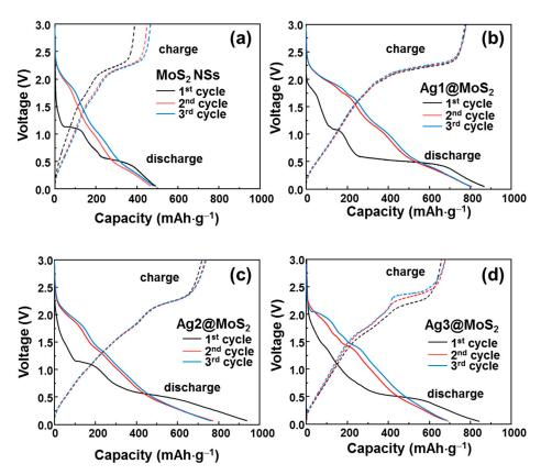
Figure 5. Initial voltage profiles of (a)  $MoS_2$  NSs, (b)  $Ag1@MoS_2$ , (c)  $Ag2@MoS_{2}$ , and (d)  $Ag3@MoS_2$  anodes.
