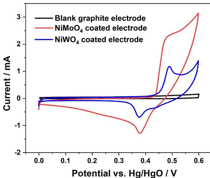
**Figure S4.** Cyclic voltammetric (CV) profile of NiMoO<sub>4</sub> and NiWO<sub>4</sub> coated on a graphite sheet. A blank graphite electrode has been compared under identical conditions to demonstrate there is no capacitance contribution. The experiment is carried out in three electrode configuration with Hg/HgO as the reference electrode at a scan rate of 2 mV/s in a 2 M NaOH solution.
