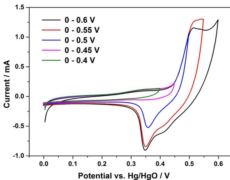
**Figure S5.** Cyclic voltammetric (CV) curves of WO<sub>3</sub> at 5mV/s in 2 M NaOH solution based on three-electrode configuration with Hg/HgO as the reference electrode with different potential window. This experiment helps us to elucidate the association between anodic and cathodic peak as the two oxidation peaks coincide and are difficult to differentiate.
