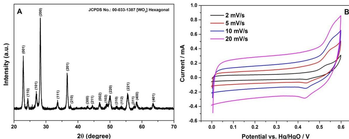
**Figure S1.** (A) X-ray diffraction (XRD) pattern of hydrothermally synthesized WO<sub>3</sub> and (B) Cyclic voltammetric (CV) curves of WO<sub>3</sub> with different scan rates in 2 M NaOH solution based on three-electrode configuration with Hg/HgO as the reference electrode.
