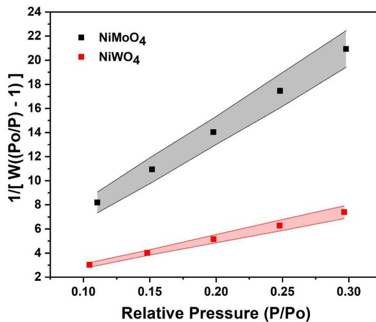
Figure S3. BET plot of NiMoO<sub>4</sub> and NiWO<sub>4</sub> using points collected at the pressure range 0.1 to 0.3.
