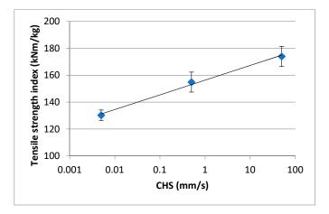
Figure 1. The effect of cross-head speed on the tensile strength of a nanocellulose film.
