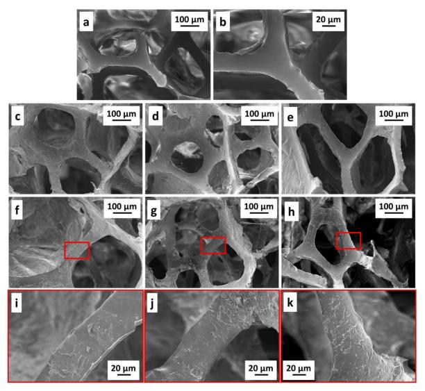
**Figure 4.** SEM micrograph of: (a) and (b) neat PU foam; 3BL (c)  $GO_A$ , (d)  $GO_B$ , (e)  $GO_C$ ; 6BL (f)  $GO_A$ , (g)  $GO_B$ , (h)  $GO_C$ ; high magnification micrograph of 6BL (i)  $GO_A$ , (j)  $GO_B$ , (k)  $GO_C$ .
