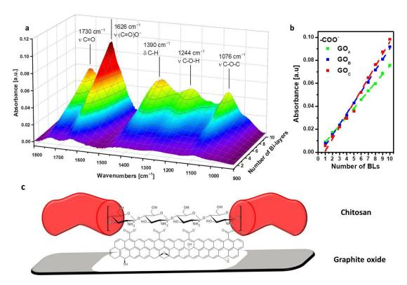
**Figure 2.** FTIR LbL growth of CHIT/GO<sub>A</sub> assembly conducted on a silicon wafer as substrate (**a**),  $1626 \text{ cm}^{-1}$  plot as function of deposited bi-layer (BL) for all the under-study assemblies (**b**), CHIT/GOx (**c**) assemblies.
