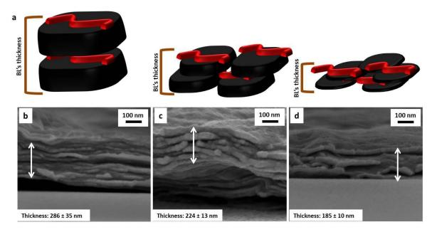
Figure 3. Schematic representation of 1BL CHIT/GO<sub>A</sub> (left), 1BL CHIT/GO<sub>B</sub> (center) and 1BL CHIT/GO<sub>C</sub> (right) thickness (a). FESEM micrograph of 10BL CHIT/GO<sub>A</sub> (b), 10BL CHIT/GO<sub>B</sub> (c), and 10BL CHIT/GO<sub>C</sub> (d) coatings on Si wafer cross-section.
