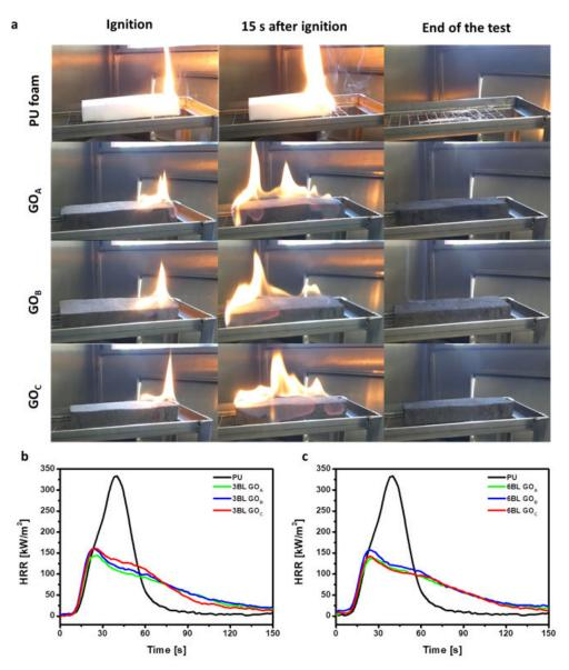
**Figure 5.** Flame retardant characterization: (a) Pictures of flammability test in horizontal configuration of untreated PU foam, 3BL CHIT/ $GO_A$  treated PU foam, 3BL CHIT/ $GO_B$  PU foam and 3BL CHIT/ $GO_C$  PU foam. First column: right after ignition, second column: 15 s after ignition and third column: end of the test. (b) HRR vs time plots of 3BL samples. (c) HRR vs time plots of 6BL samples.
