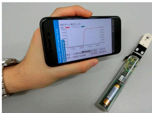
**Figure 17.** Portable biosensing system using a Bluetooth connection between a smartphone and the field-effect transistor-based biosensor. Reproduced with permission from [131].
