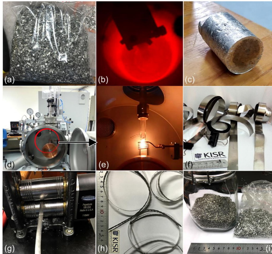
Figure 1. Conversion of solid-waste (SW) Mg machining chips into microscaled Mg-shots. (a) as-received SW-Mg chips, (b) melting and casting processes, (c) as-casted pure (99.95 wt%) Mg-ingot, (d), (e) melt spinning (MS) process, (f) as-MS Mg-ribbons, (g) cold rolling (CR) process, (h) as-CR Mg-strips, and (i) as-snipped Mg-shots.
