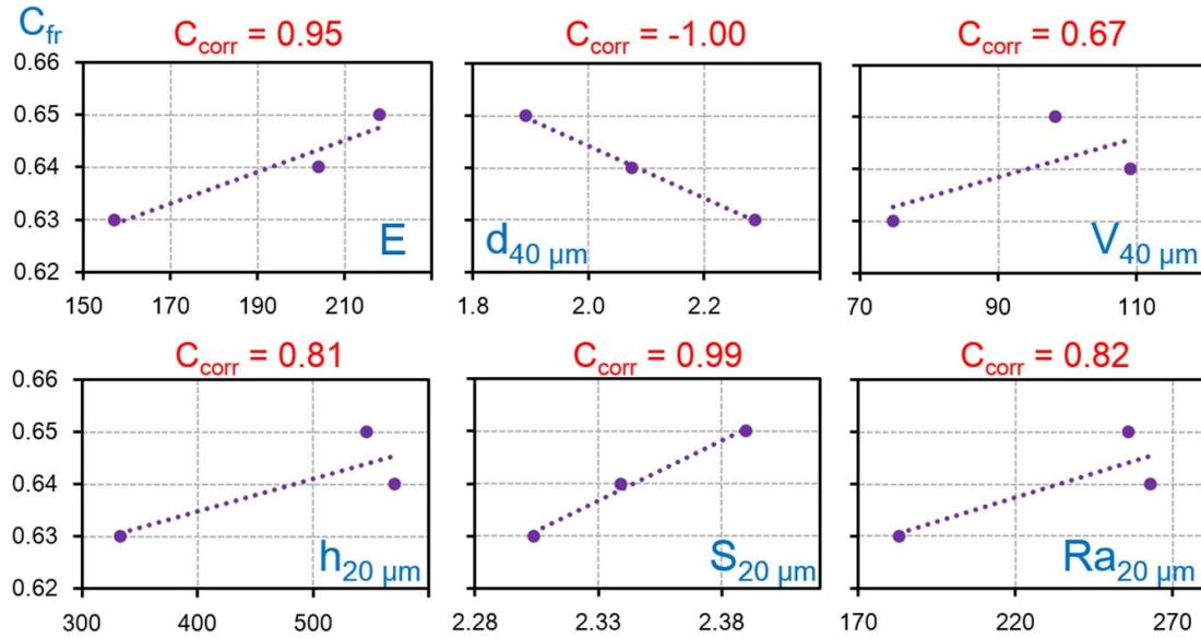
**Figure S6.** The correlation coefficients between  $C_{fr}$  and  $E$  and particles characteristics for AlCrN coatings.
