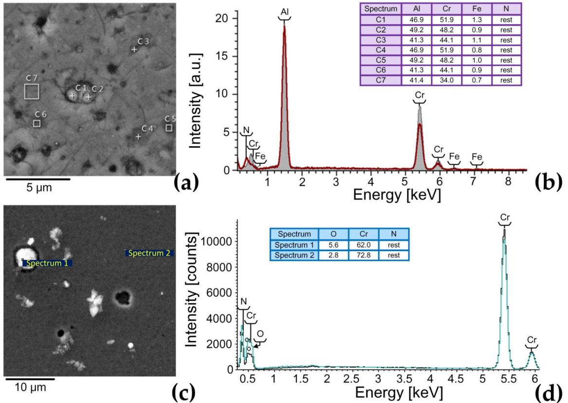
**Figure S1.** SEM images and spectra of microparticles and surface in Al<sub>70</sub>Cr<sub>30</sub>N and CrO(5)N coatings: (a,c): image; (b,d): spectrum and table with the elements content; (a):Al<sub>70</sub>Cr<sub>30</sub>N, ×10000; (d): CrO(5)N, ×5000.
