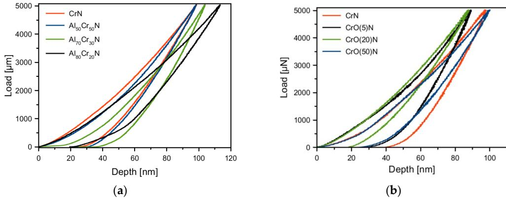
**Figure S3.** The NI completely load/unload curves in AlCrN coatings (a) and in CrON coatings (b).
