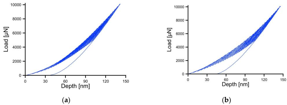
**Figure S4.** The NI progressive partial load/unload curves with partial unloading of CrN (a) and Al<sub>50</sub>Cr<sub>50</sub>N (b) coatings.
