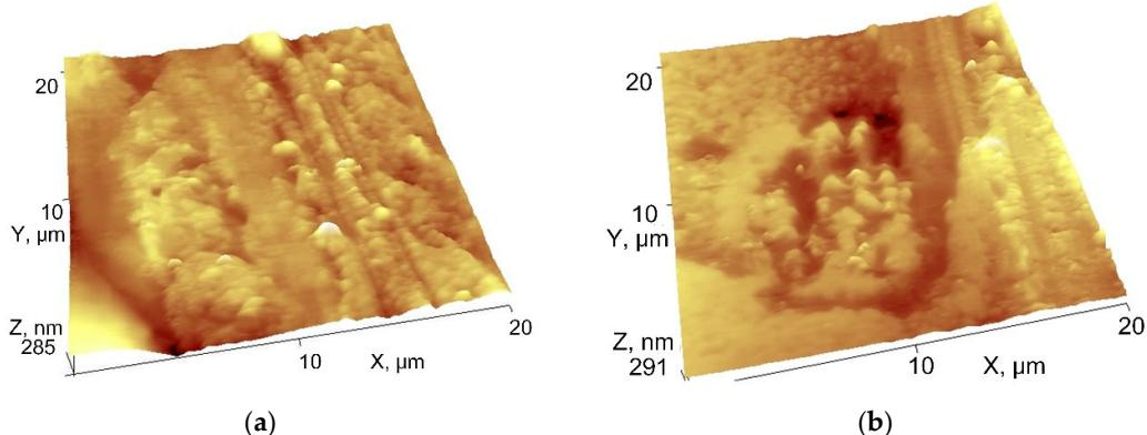
**Figure S5.** The upper modified layer formed under tribological load on the CrN (a) and CrO(50)N (b) coatings surface, area of 20 × 20 μm<sup>2</sup>.
