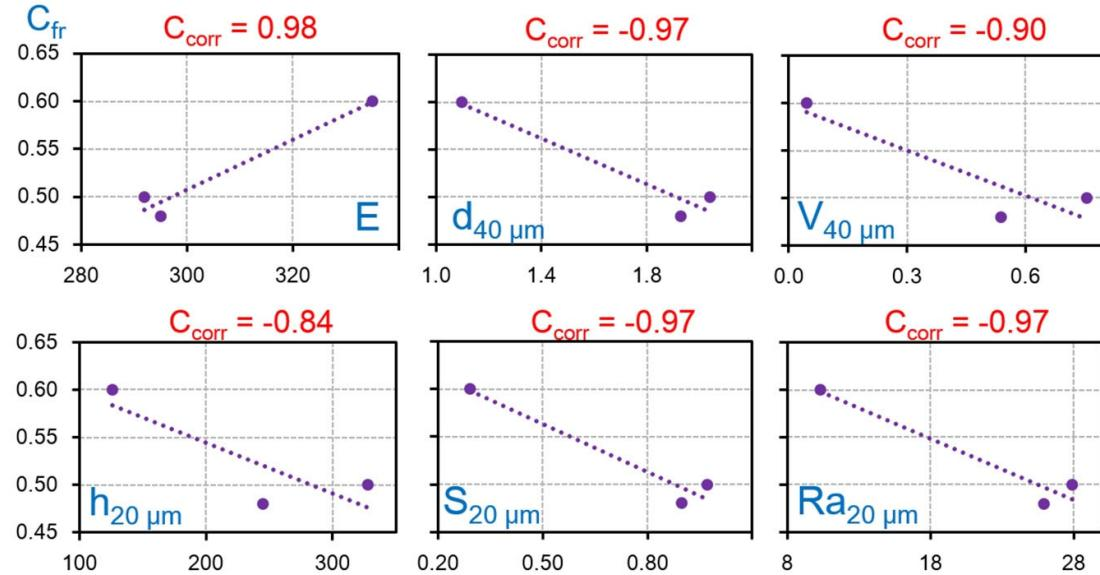
**Figure S7.** The correlation coefficients between  $C_{fr}$  and  $E$  and particles characteristics for CrON coatings.
