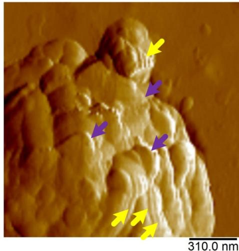
**Figure S2.** AFM image with the layered microstructure of microparticle from Figure 4a. Examples of layers are marked with violet; sublayers are marked with yellow.
