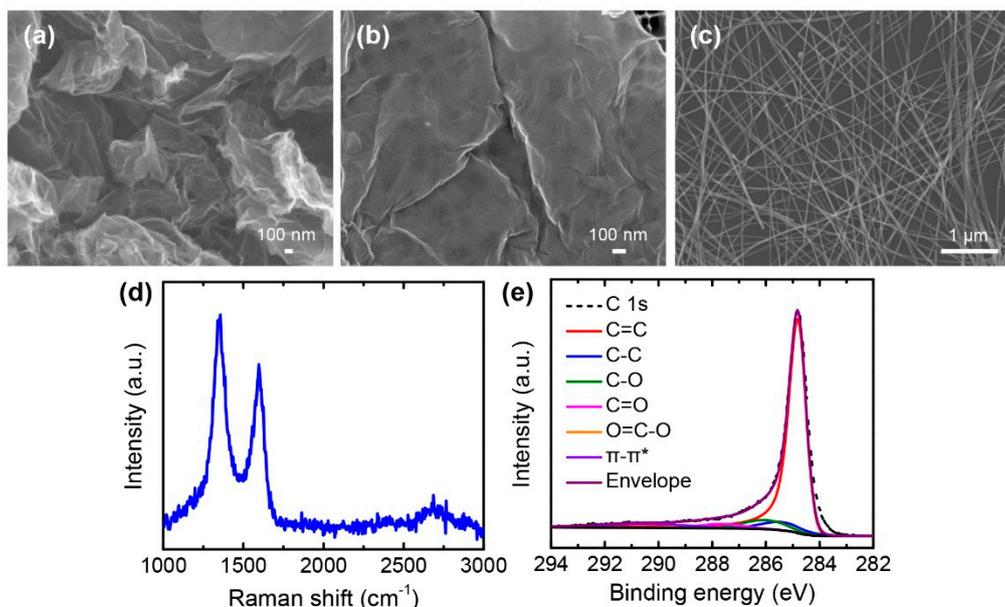
**Figure 1.** Characterization of reduced graphene oxide (rGO) and silver nanowires (AgNWs). (a,b) Scanning electron microscopy (SEM) images of: (a) as-received rGO powders; (b) Sonicated rGO powders; (c) SEM image of AgNWs placed on a silicon substrate; (d) Raman spectrum of as-received rGO powders; (e) X-ray photoelectron spectroscopy (XPS) C 1s core-level spectra of as-received rGO powders.
