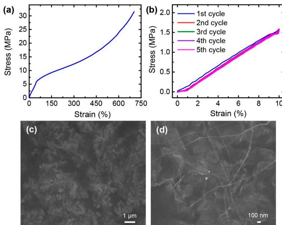
**Figure 2.** (a) Stress–strain curve of the neat spandex film; (b) Stress–strain curves of the neat spandex film under stretching and releasing cycles with a strain of 10%; (c,d) SEM images of the surfaces of: (c) Graphene/spandex (G/SpX); (d) Graphene/AgNW/spandex (G/AgNW/SpX) composite films.
