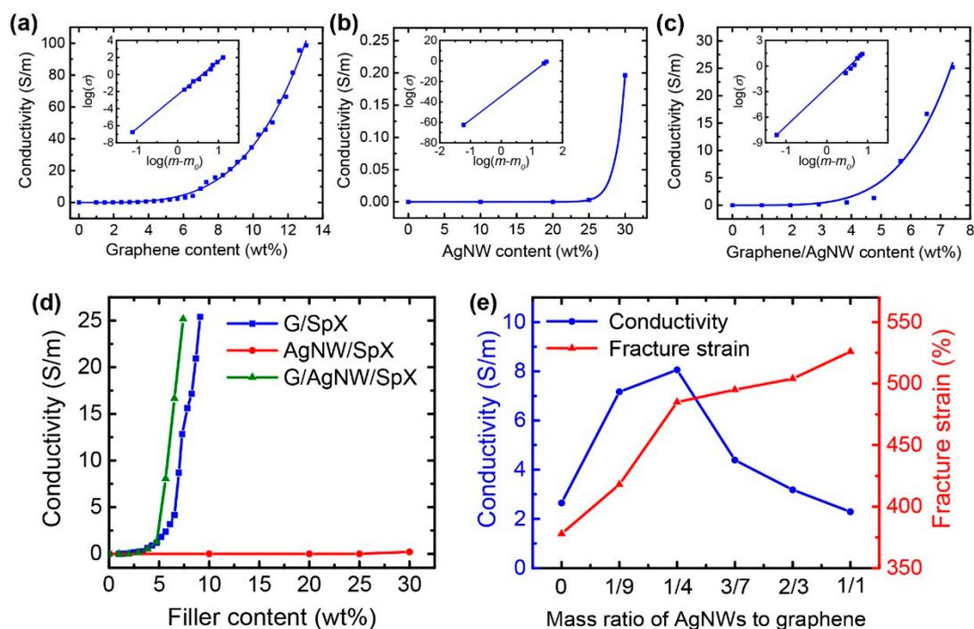
**Figure 3.** (a–d) Electrical conductivity of composite films as a function of filler loading; The insets in (a–c) show the  $\log(\sigma)$  versus  $\log(m - m_0)$ ; The G/AgNW/SpX composite in (c) had a mass ratio of AgNWs to graphene of 1/4; (d) Comparison of the electrical conductivity of composite films; (e) Electrical conductivity and fracture strain of the G/AgNW/SpX composite as a function of the mass ratio of AgNWs to graphene, with a total filler concentration of 5.66 wt%.
