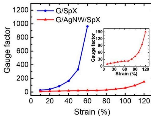
**Figure 6.** GFs of the G/SpX and G/AgNW/SpX composite strain sensors. The inset shows the detailed GF of the G/AgNW/SpX sensor.
