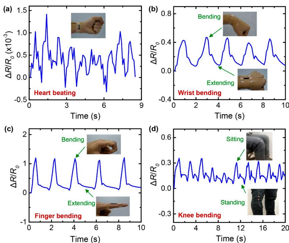
**Figure 9.** Real-time monitoring of various human motions using stretchable G/AgNW/SpX composite strain sensors. Resistance responses of the sensors clearly indicate: (a) heartbeats at the wrist; (b) bending of the wrist; (c) bending of the finger; (d) movement of the knee joint.
