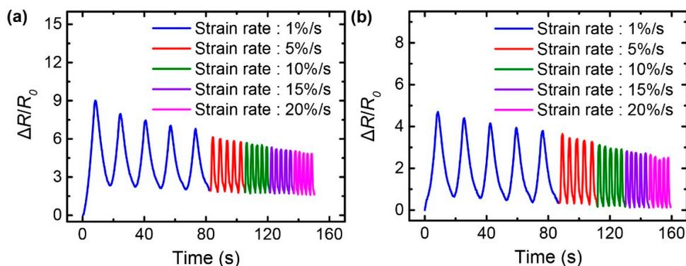
**Figure 8.** Resistance-strain responses of the: (a) G/SpX; (b) G/AgNW/SpX composite strain sensors at various strain rates, with a strain of 10%. The pre-strain of 10% was applied to the sensors.
