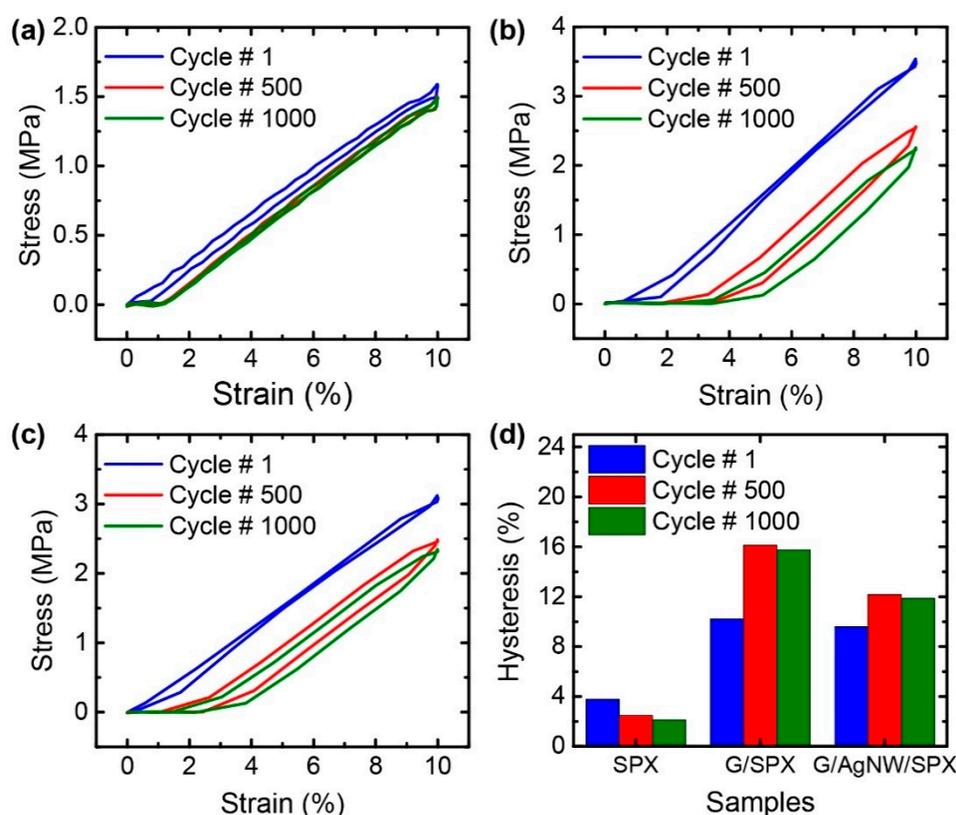
**Figure 4.** (a–c) Stress–strain curves of: (a) neat spandex; the (b) G/SpX; (c) G/AgNW/SpX films during the 1st, 500th, and 1000th cycles; (d) Mechanical hysteresis ( $H_M$ ) obtained from the stress–strain curves for each film.
