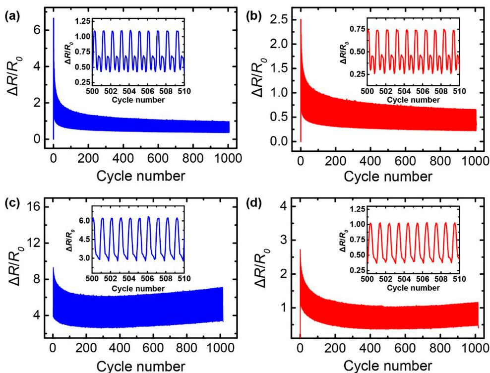
**Figure 7.** Resistance-strain responses of the: (a,c) G/SpX; (b,d) G/AgNW/SpX composite strain sensors under 1000 stretching–releasing cycles with a strain of 10%; (a,b) Without pre-strain; (c,d) With 10% pre-strain. The insets show the detailed responses of the sensors.
