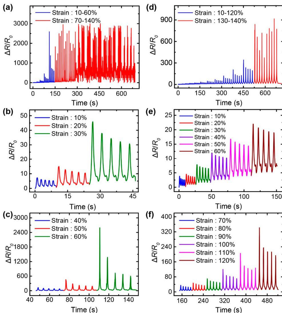
**Figure 5.** Resistance responses of the: (a–c) G/SpX; (d–f) G/AgNW/SpX composite strain sensors under various strain levels; (a,d) Relative change in resistance of the sensors at strains ranging from 10- to 140%; (b,c,e,f) Detailed resistance-strain responses of the sensors at each strain level.
