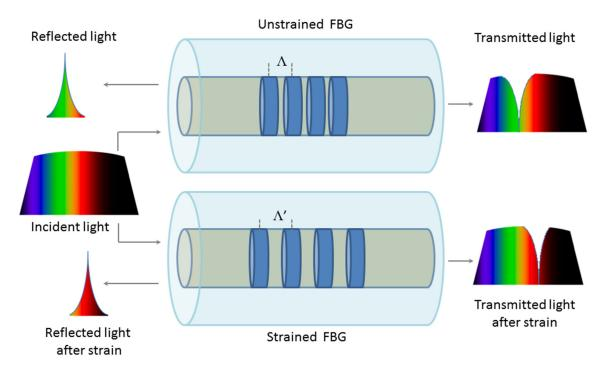
**Figure 1.** Schematic of the working principle of Fiber Bragg grating (FBG) sensors, and its response to strain.
