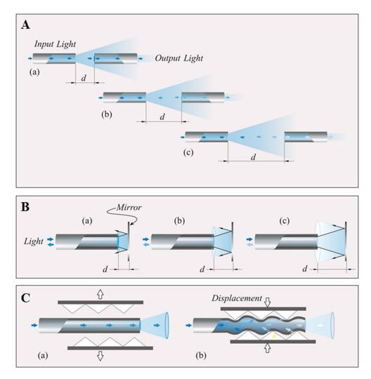
**Figure 2.** (**A**) Schematic of the working principle of an intensity modulated sensor using two fiber optic; (**B**) schematic of the working principle of an intensity modulated sensor using a fiber optic and a mirror; (**C**) schematic of the light lost from the fiber core caused by bending (adapted from [10]).
