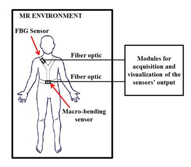
**Figure 3.** Schematic representation of the monitoring systems proposed by and developed in the optical fiber sensors embedded into technical textile for healthcare (OFSETH) project.
