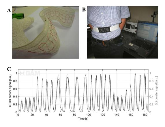
**Figure 5.** (**A**) Textiles based on macrobending FOS embedding a standard single mode fiber (adapted from [57]); (**B**) Macrobending sensors for monitoring of abdominal movements (adapted from [57]); (**C**) Output of the OTDR sensors during the monitoring of abdominal movement (adapted from [57]).
