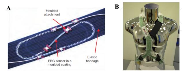
**Figure 4.** (**A**) Design of the FBG sensor developed in OFSETH project (adapted from [57]); (**B**) MRI-compatible sensing harness which embeds the fiber optic sensors for respiratory monitoring (adapted from [57]).
