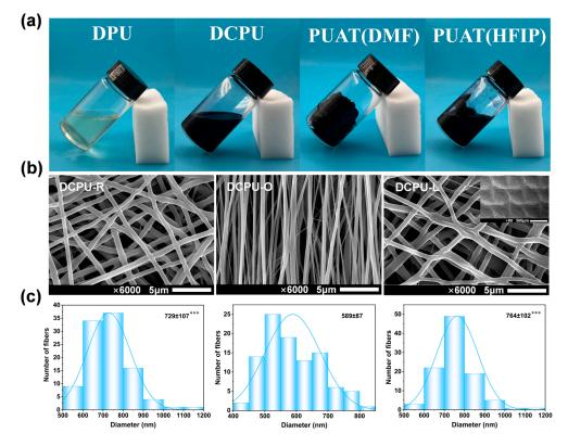
**Figure 3.** Dissolvability, processibility of copolymers and topological structure of scaffolds: (**a**) Digital photos of the dissolution state of copolymers in solvents; (**b**) Surface topological structure of DCPU fibrous scaffolds; (**c**) Fibers' diameter of fibrous networks with three different surface topological structure. \*\*\* p < 0.001 statistically significant compared with DCPU-O (n = 100).
