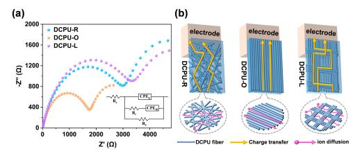
**Figure 4.** Electrochemical properties of the DCPU fibrous networks: (**a**) Nyquist plot and equivalent circuit model obtained from the EIS characterization of fibrous networks with three patterns, (**b**) schematic illustration of the charge transfer and ion diffusion pathways through fibrous networks with three patterns.
