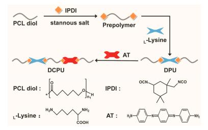
Figure 1. Synthesis route of DPU and DCPU copolymers (\*: the repeat unit of PCL-diol).
