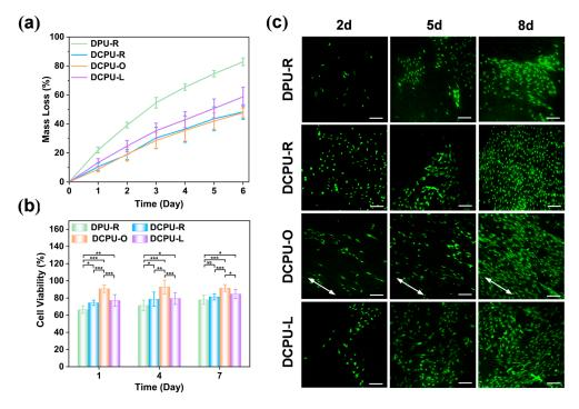
**Figure 5.** In vitro biodegradability and cytocompatibility of fibrous scaffolds: (**a**) in vitro degradation profiles immersed in lipase solution (n = 5); (**b**) CCK-8 analysis of BMSCs cultured on DPU-R and DCPU fibrous scaffolds on day 1, 4, and 7 days (\* p < 0.05, \*\* p < 0.01, \*\*\* p < 0.001) (n = 3); (**c**) Live cell fluorescence staining images of BMSCs seeded on DPU-R and DCPU fibrous scaffolds on day 2, 5, and 8 days. Scale bar: 100 µm. Arrows: cell orientation.
