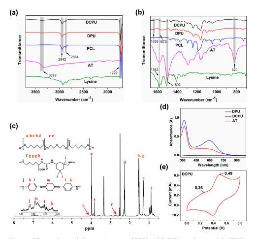
**Figure 2.** Physicochemical characterizations of DPU and DCPU copolymers: (**a**,**b**) FT-IR spectra of the DPU and DCPU copolymers and their raw materials in different wave band, (**c**) <sup>1</sup>H NMR spectrum of the DCPU copolymer (the different letters represented the correspondence between chemical structure of materials and peaks in the <sup>1</sup>H NMR), (**d**) UV–vis spectra of AT, DPU, and DCPU dispersed in DMF, (**e**) Cyclic voltammogram of DCPU copolymer in 1 M HCl.
