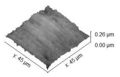
**Figure 9.** Three-dimensional  $45 \times 45 \ \mu\text{m}^2$  TM-AFM image of region 1 after bending. The z-range is 320 nm from black to white.
