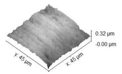
Figure 7. Three-dimensional 45  $\times$  45  $\mu m^2$  TM-AFM image of region 1 before bending. The z-range is 320 nm from black to white.
