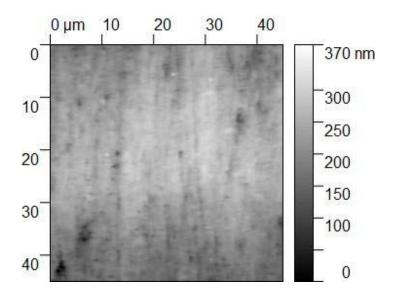
Figure 6. The 45  $\times$  45  $\mu m^2$  TM-AFM image of region 1 before bending. The z-range is 370 nm from black to white.
