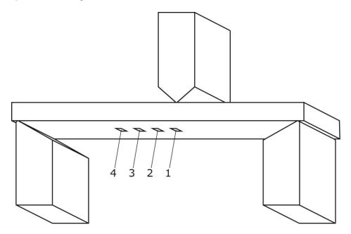
Figure 3. Schematic illustration of the three-point flexure test setup and the regions for AFM analysis.
