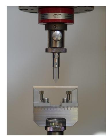
Figure 4. Three-point flexure test setup.
