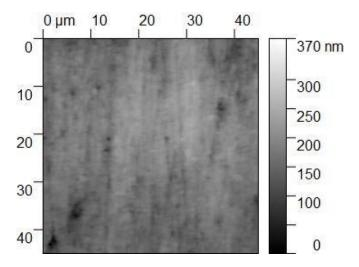
Figure 8. The 45  $\times$  45  $\mu m^2$  TM-AFM image of region 1 after bending. The z-range is 320 nm from black to white.
