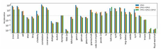
**Figure 5.** Acceleration of the Polybench/C suite algorithms by the proposed platform, using the largest data size allowed by the capabilities of the computing devices employed: CPU1 (Intel i9-9920X), GPU1 (Nvidia Quadro P5000), and GPU2 (Nvidia GeForce GT 710).
