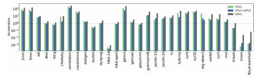
**Figure 6.** Acceleration of the Polybench/C suite algorithms by the platform, using the largest data size allowed by the computing devices employed: CPU1 (Intel i9-9920X) and GPU1 (Nvidia Quadro P5000).
