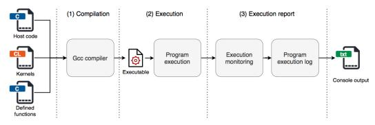
Figure 4. Task sequence of the program execution module.
