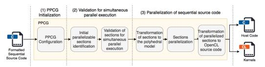
Figure 3. Algorithm deployment module task sequence.
