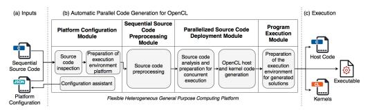
Figure 1. Architecture of the proposed heterogeneous computing platform; general and flexible.
