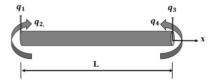
Figure 2. The Timoshenko beam element.
