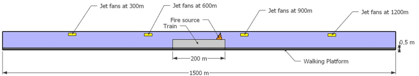
**Figure 1.** Side sketch of the tunnel with dimensions, the jet fans’ placement along the tunnel at positions  $x = 300, 600, 900,$  and  $1200$  m, and the walking platform.
