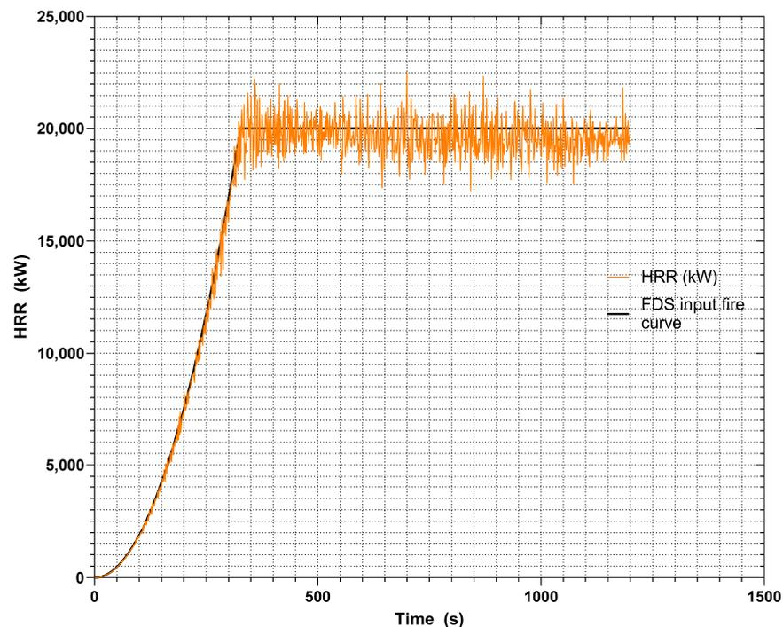
**Figure 3.** Input fire ramp curve and numerical results.
