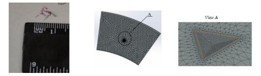
Figure 10. Actual defect and calculation grid for a defect on a disc segment.
