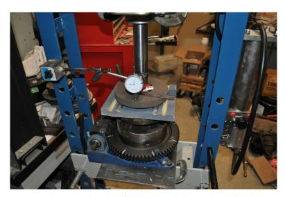
Figure 2. Three-point bending fixture to crack the grinding wheels.
