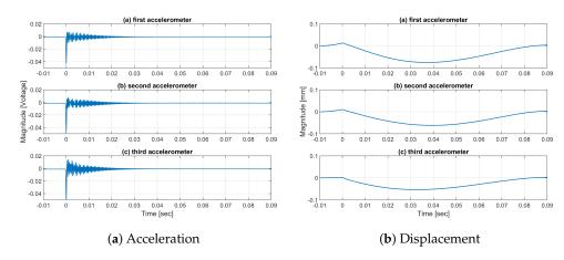
Figure 12. Typical acceleration and displacement results of the 25 mm glued 120 grit wheel.
