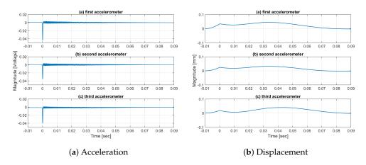
Figure 7. Typical acceleration and displacement of the new 60 grit wheel.
