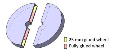
Figure 3. Glued segments of the grinding wheel.
