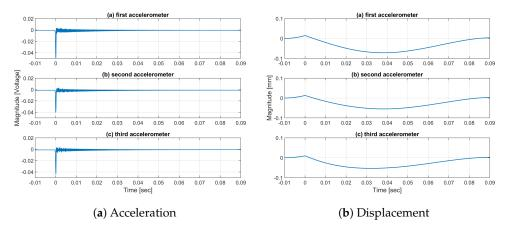
Figure 11. Typical acceleration and displacement results of the fully glued 120 grit wheel.
