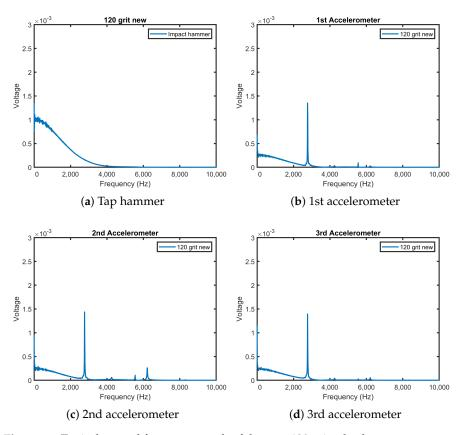
Figure 16. Typical natural frequency result of the new 120 grit wheel.
