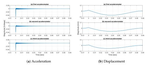
Figure 8. Typical acceleration and displacement results of the fully glued 60 grit wheel.
