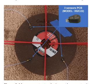
Figure 5. Measurement setup for impact hammer testing.
