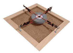
Figure 4. Test fixture to suspend the grinding wheel.
