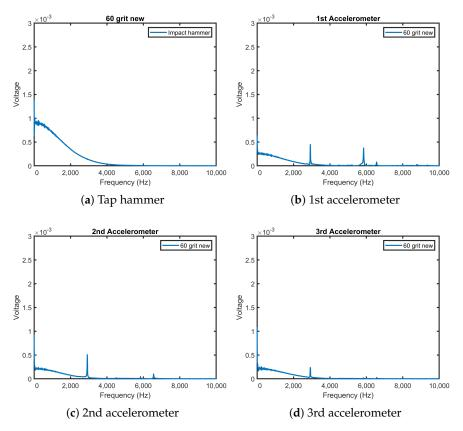
Figure 13. Typical natural frequency result of the new 60 grit wheel.
