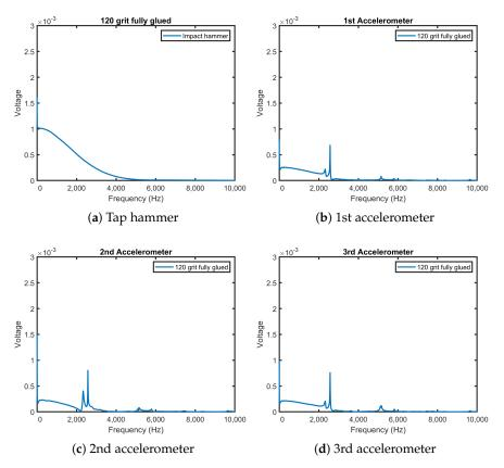
Figure 17. Typical natural frequency result of the fully glued 120 grit wheel.
