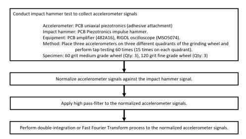
Figure 6. Accelerometer signal processing procedure.
