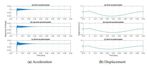
Figure 9. Typical acceleration and displacement results of the 25 mm glued 60 grit wheel.
