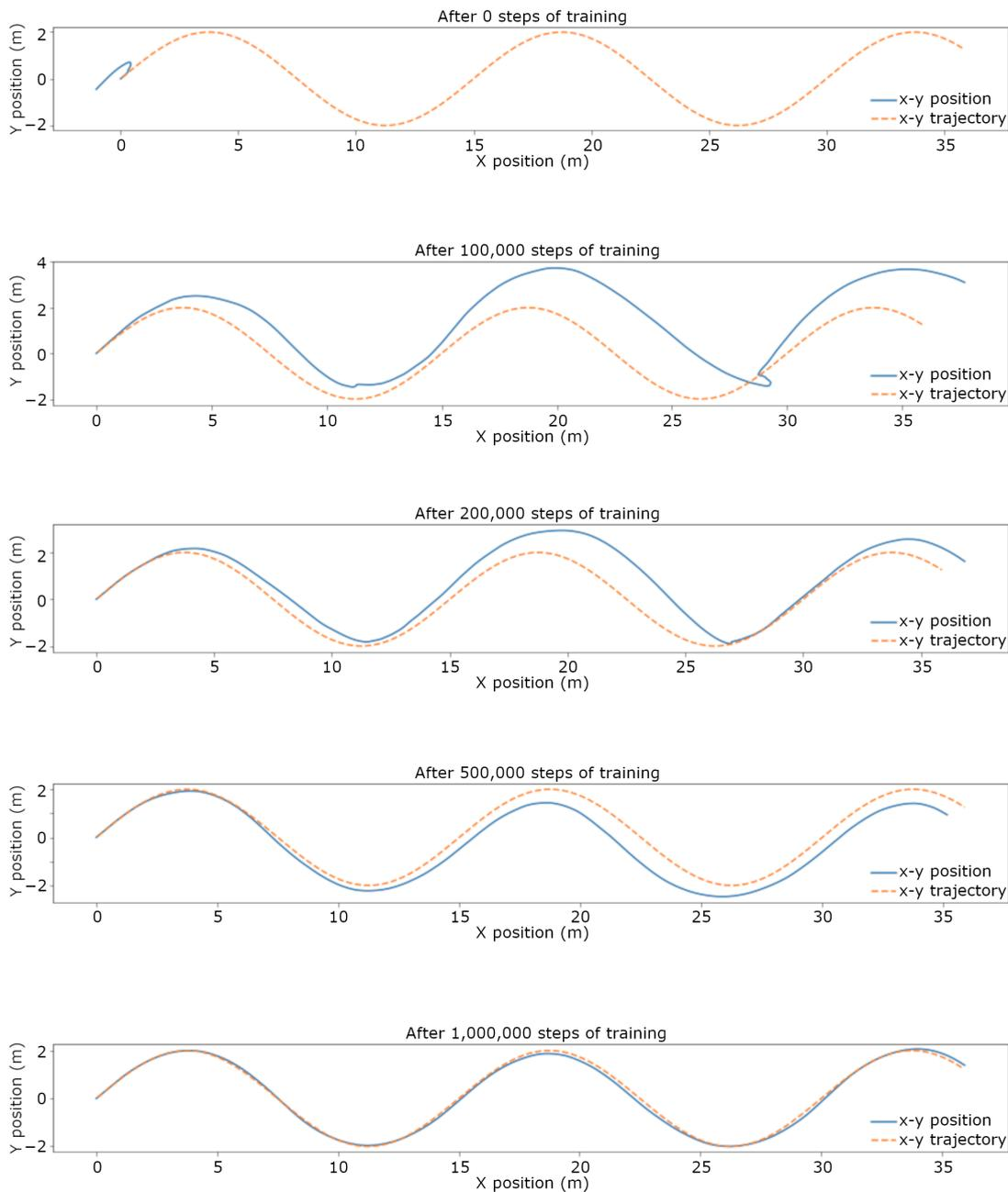
**Figure 6.** Visualization of intermediate trajectory tracking training results for the RL controller upon initialization: 100,000, 200,000, 500,000, and 1,000,000 training steps.
