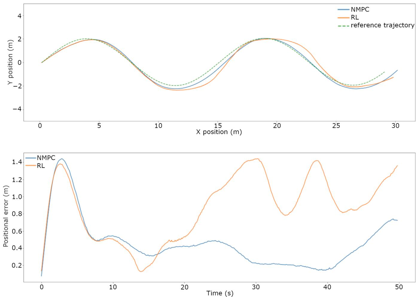
**Figure 15.** Scenario 5—real world. Comparison between the NMPC and RL algorithm trajectory tracking performance on the real Roboat vessel. Trajectories of NMPC, RL, and reference sine wave on the top; tracking errors of NMPC and RL on the bottom.
