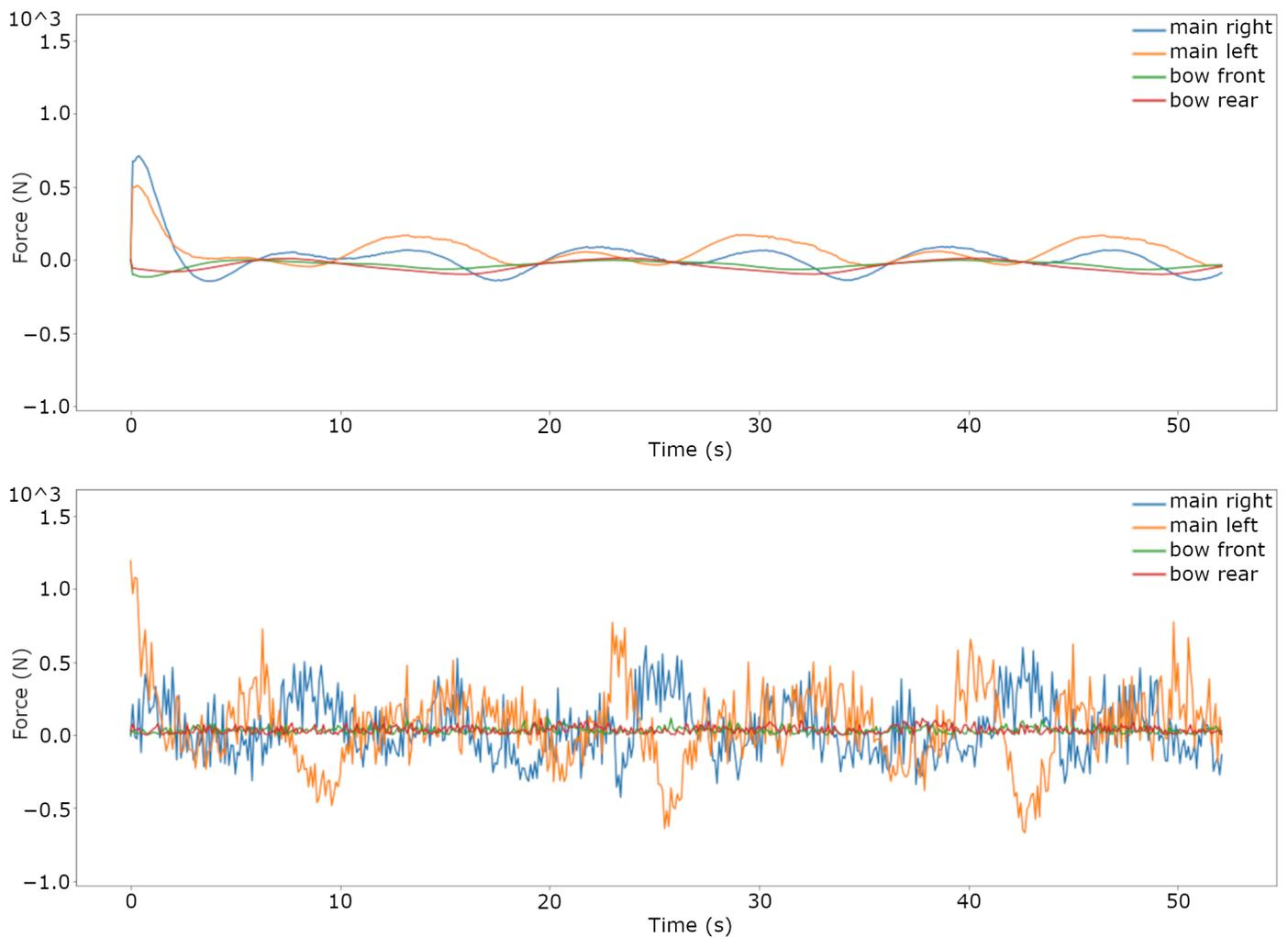
**Figure 14.** Scenario 4—wind. Comparison between the NMPC and RL algorithm trajectory tracking performance with a wind of speed 9 m/s acting on the system. Force allocation of NMPC (**top graph**) and RL (**bottom graph**) for tracking the sine wave trajectory.
