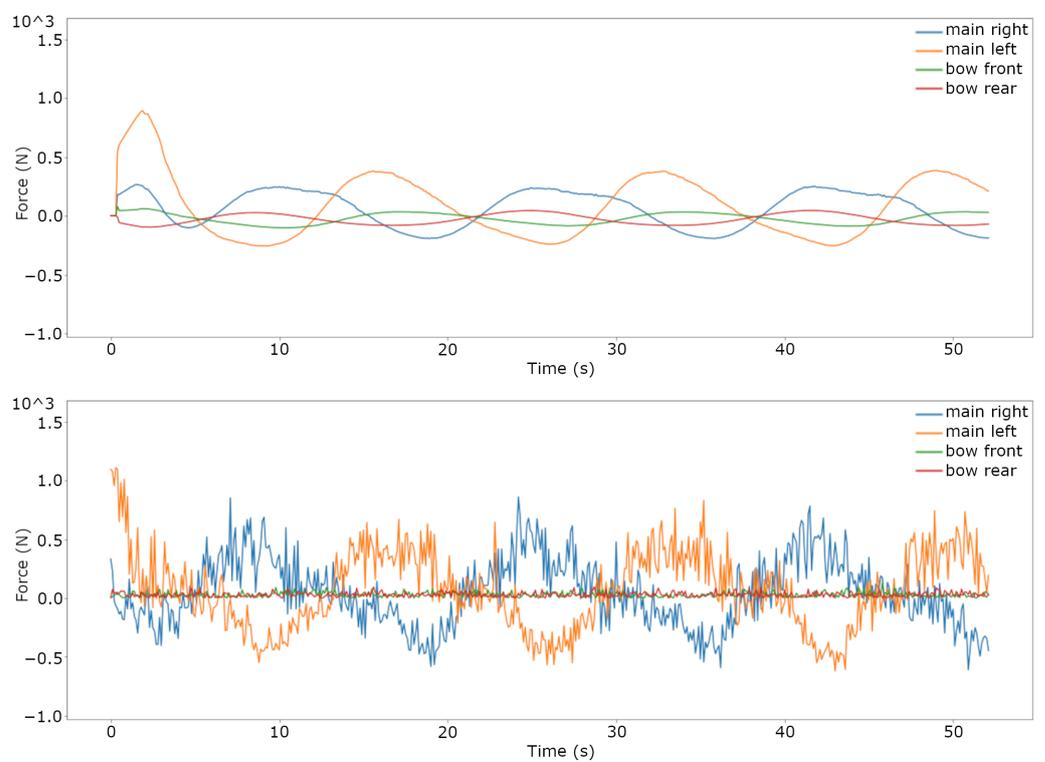
**Figure 12.** Scenario 3—current. Comparison between the NMPC and RL algorithm trajectory tracking performance with a current of 0.5 m/s acting on the system. Force allocation of NMPC (top graph) and RL (bottom graph) for tracking the sine wave trajectory.
