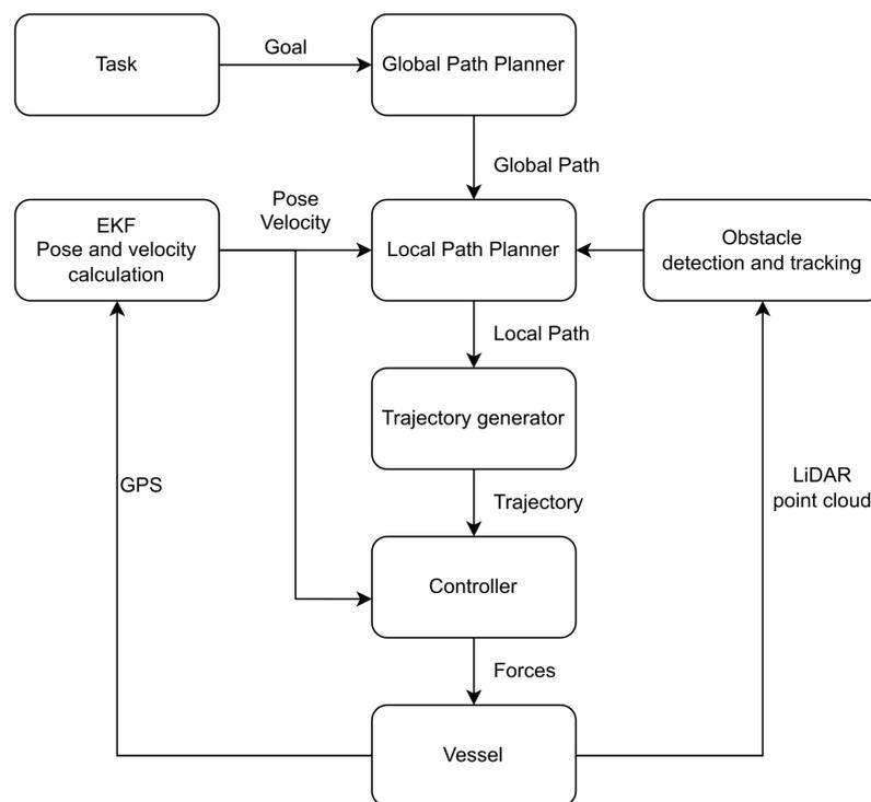
**Figure 2.** Structure of the Roboat platform architecture.
