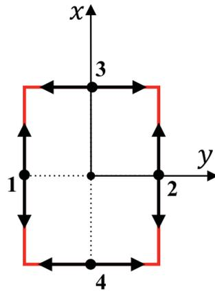
Figure 1. Roboat platform “+” thruster configuration.
