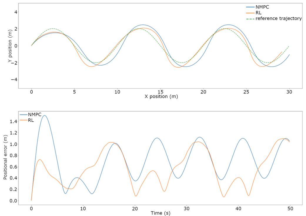
**Figure 9.** Scenario 2—payload. Comparison between the NMPC and RL algorithm trajectory tracking performance with payload equal to 50% of vessel’s mass. Trajectories of NMPC, RL, and reference sine wave on the top graph. Tracking errors of NMPC and RL on the bottom graph.
