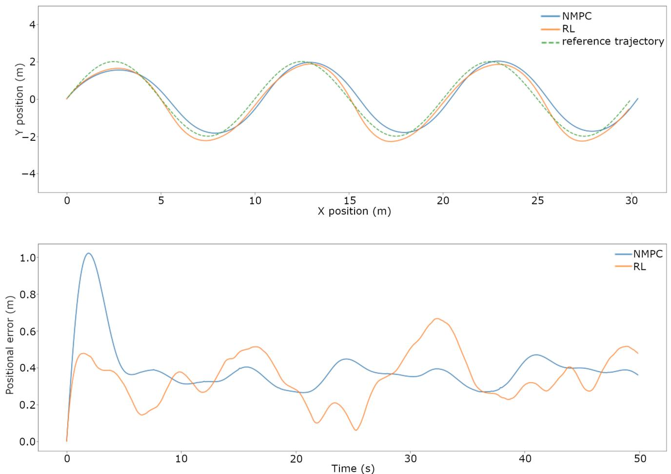
**Figure 7.** Scenario 1—baseline. Comparison between the NMPC and RL algorithm trajectory tracking performance. Trajectories of NMPC, RL, and reference sine wave on the top graph. Tracking errors of NMPC and RL on the bottom graph.
