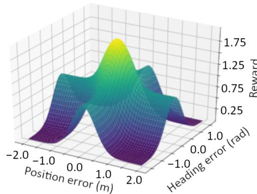
Figure 3. Visualization of Gaussian terms in the reward function in a 3D plot.
