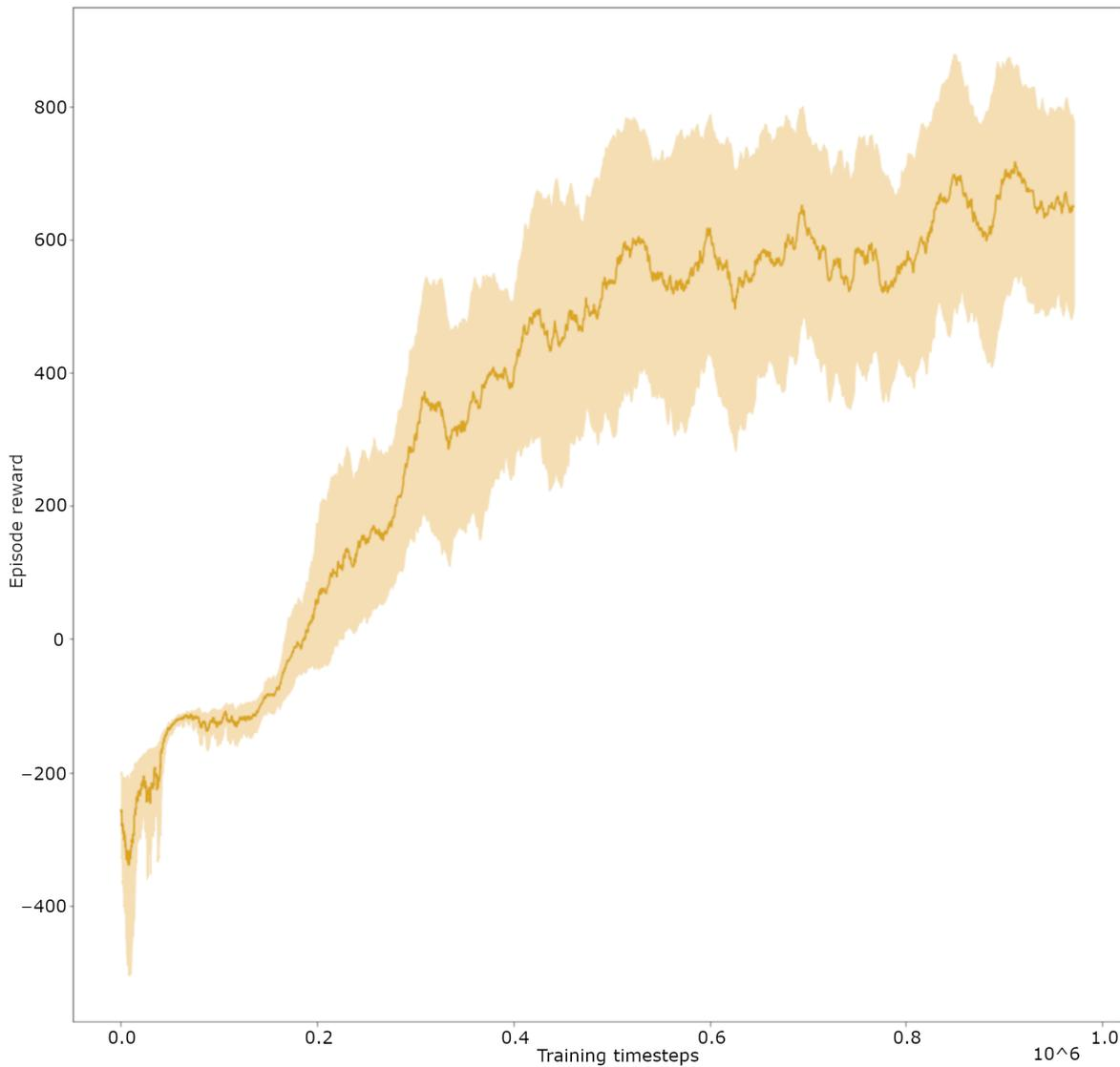
**Figure 5.** Plot of the episodic reward throughout one million steps of training. Orange line presents the moving average with a window size 50; light orange presents the standard deviation of the value.
