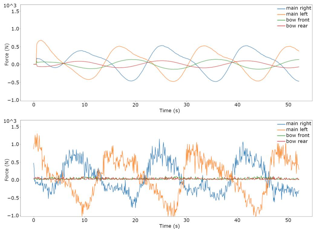
**Figure 10.** Scenario 2—payload. Comparison between the NMPC and RL algorithm trajectory tracking performance with payload equal to 50% of vessel’s mass. Force allocation of NMPC (top graph) and RL (bottom graph) for tracking the sine wave trajectory.
