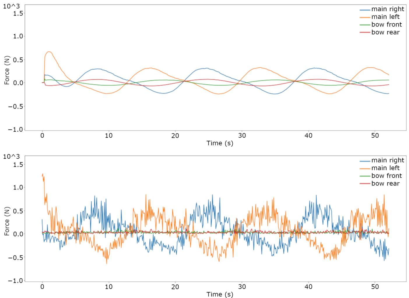
**Figure 8.** Scenario 1—baseline. Comparison between the NMPC and RL algorithm trajectory tracking performance. Force allocation of NMPC (top graph) and RL (bottom graph) for tracking the sine wave trajectory.
