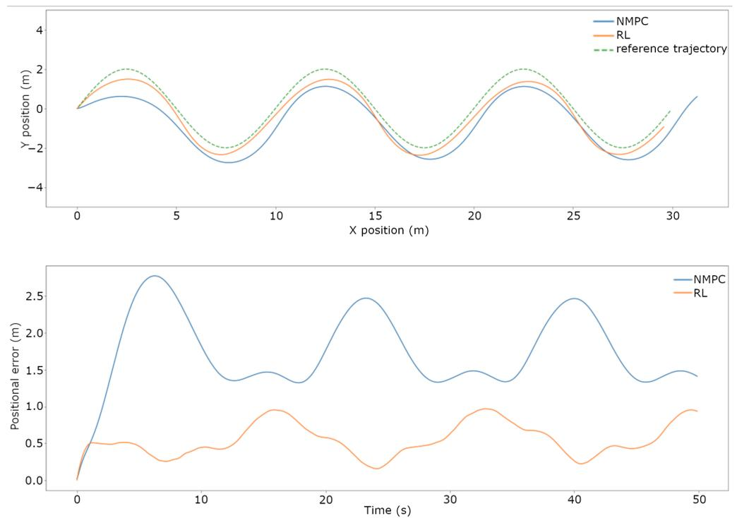
**Figure 11.** Scenario 3—current. Comparison between the NMPC and RL algorithm trajectory tracking performance with a current of 0.5 m/s acting on the system. Trajectories of NMPC, RL, and reference sine wave on the top graph. Tracking errors of NMPC and RL on the bottom graph.
