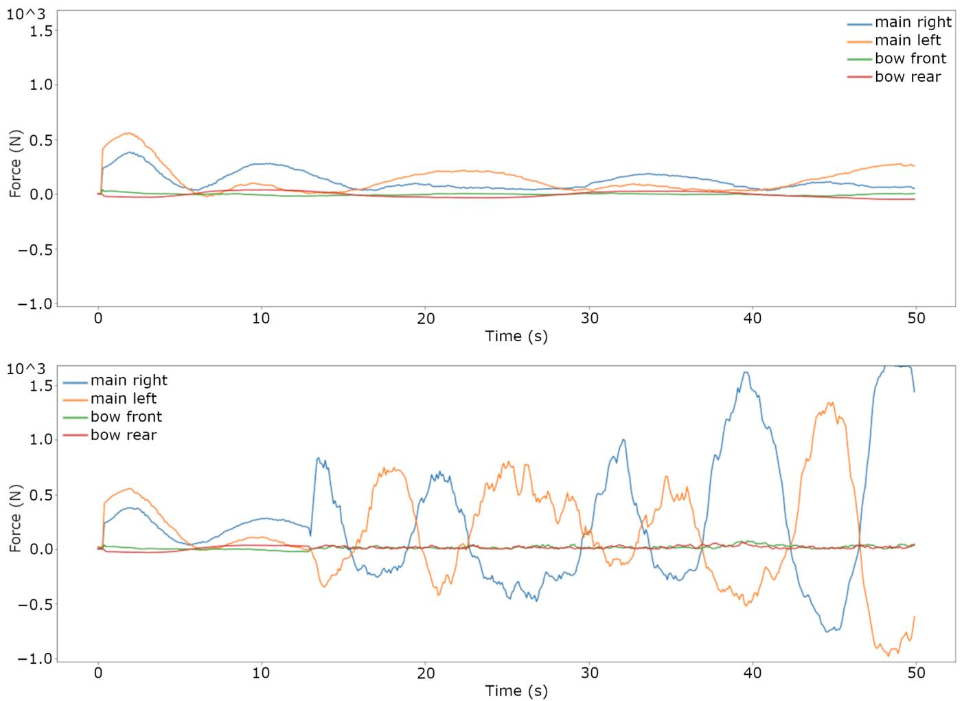
**Figure 16.** Scenario 5—real world. Comparison between the NMPC and RL algorithm trajectory tracking performance on the real Roboat vessel. Force allocation of NMPC (**top graph**) and RL (**bottom graph**).
