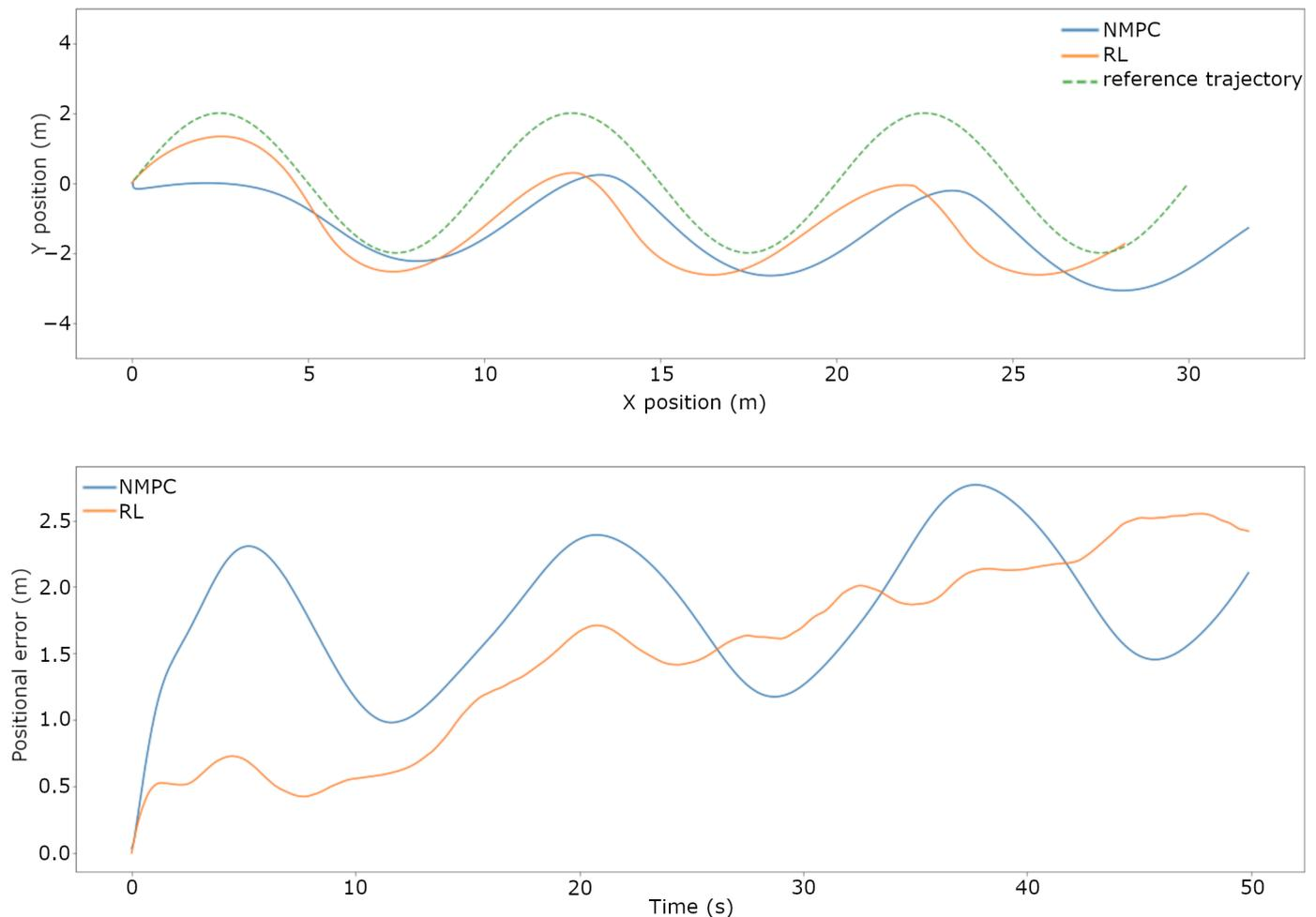
**Figure 13.** Scenario 4—wind. Comparison between the NMPC and RL algorithm trajectory tracking performance with a wind of speed 9 m/s acting on the system. Trajectories of NMPC, RL, and reference sine wave on the top graph. Tracking errors of NMPC and RL on the bottom graph.
