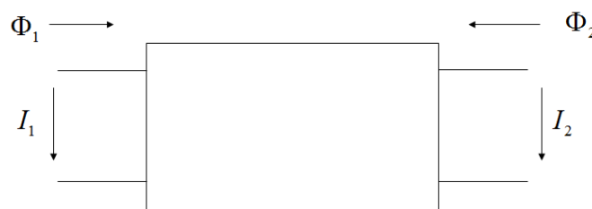
Figure 2. Information gate ( \Phi —information flow of data measured in bits per second, I —information content measured in Joules per bit).
