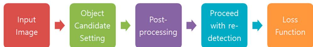
Figure 4. Hybrid human detection 4-step workflow.
