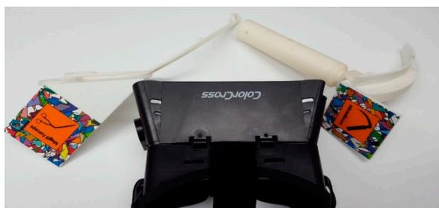
**Figure 6.** Three-dimensional printed tools with AR image targets, including a ColorCross head mount for mobile phone simulation [12].
