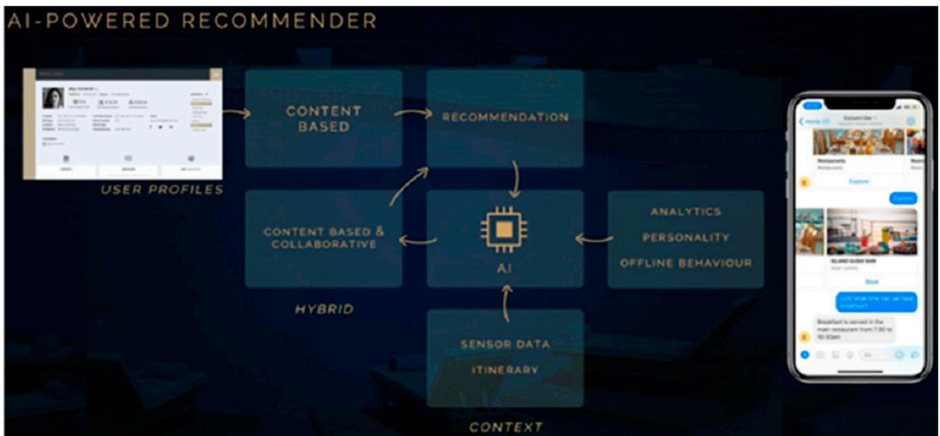
Figure 2. The structure of eXclusivi’s recommendation system.
