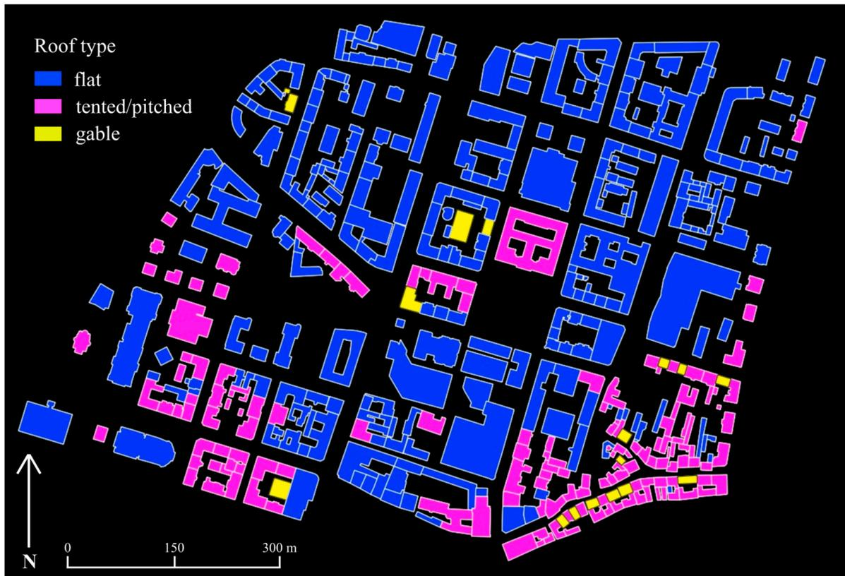
Figure 7. Roof types in the analyzed area.
