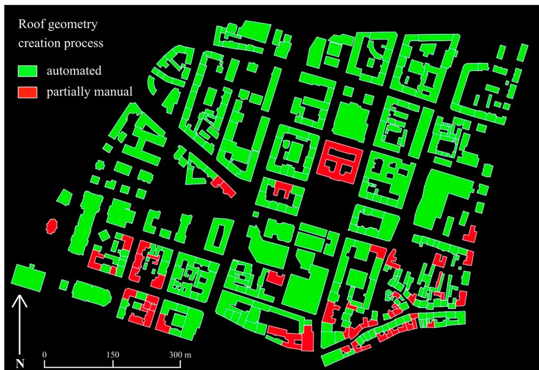
Figure 19. Coverage of buildings with automatically generated roof geometry (green) and roof geometries with manual improvement needed (red).
