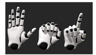
**Figure 2.** The three different hands poses tracked by the system: open hand (**left**), grab pose (**center**), and pointing pose (**right**).
