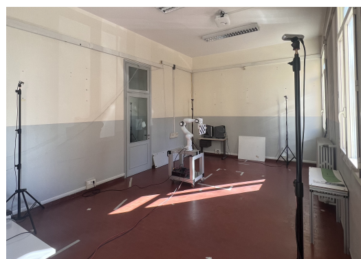
Figure 4. Large-scale real workcell equipped with a Panda robot arm with a checkerboard attached on its end-effector, surrounded by four Intel RealSense Depth D455 cameras.
