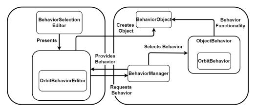
Figure 5. Object movement behavior tool's architecture.
