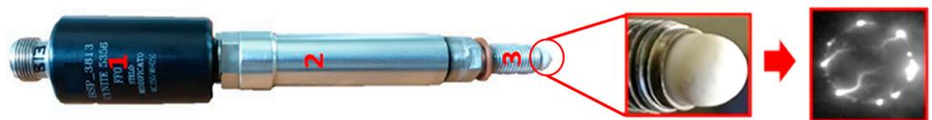
Figure 2. Tested igniter (left) (1 = inductor, 2 = connection, 3 = firing end) and corresponding firing end detail (middle). Discharge event (right): ionization waves (i.e., streamers) propagated above the igniter cupola.
